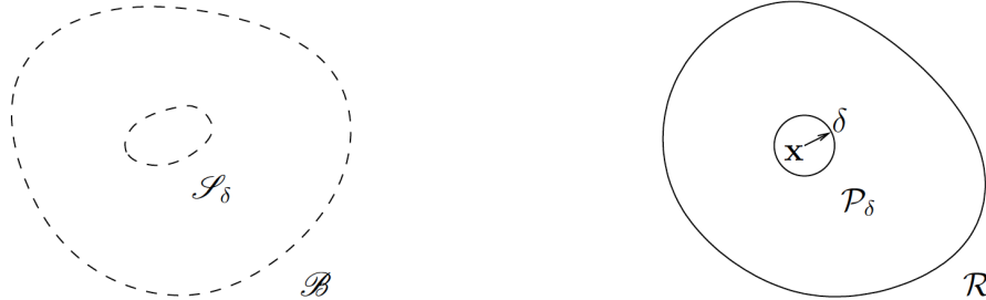
Figure 2.3: A limiting process used to define the mass density \rho at a point \mathbf{x} in the current configuration [43]
