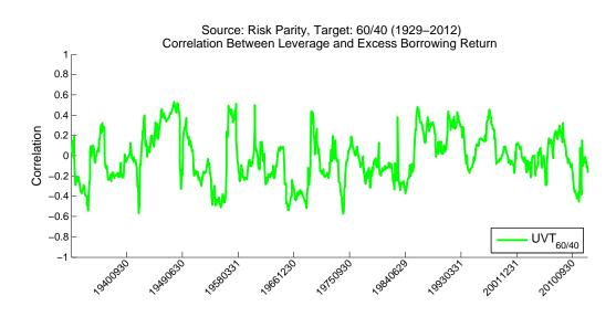
Correlation of excess borrowing return and leverage for  $UVT_{60/40}$ , risk parity levered to match the realized volatility of 60/40 fixed mix over the period 1929–2012. Correlation was computed from monthly data using a trailing 36-month window.
