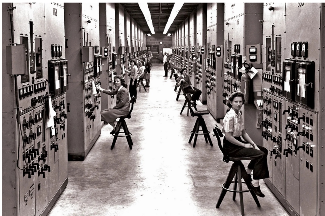
Women employees of the Manhattan Project operate calutron control panels at Y-12, in a US government photo by Ed Westcott.
