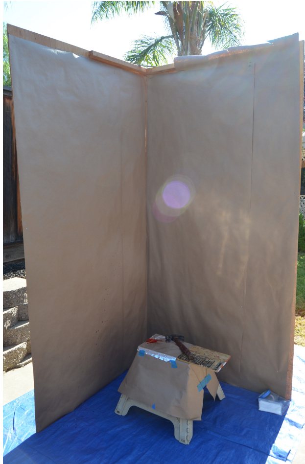
Figure 4: Set up for point of origin experiments. Constructed walls covered in brown paper packaging with stand where blood is struck to create a spatter pattern. The left wall was the north/main wall, and the right was the east/west wall. From experiment number 3.
