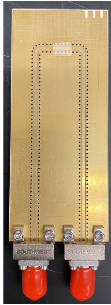
Figure 3.12: A U-shaped transmission line for inductive measurements.
