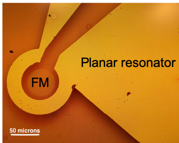
Figure 6.5: The YIG micro-disks inside the \Omega -shaped planar resonator micro-coil before the thermal annealing.
