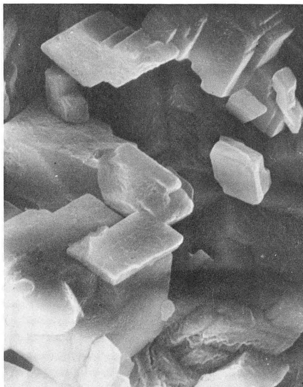
Figure 2. SEM picture of the \text{CaO} particles produced by complete decomposition of the \text{CaCO}_3 of Figure 1.
