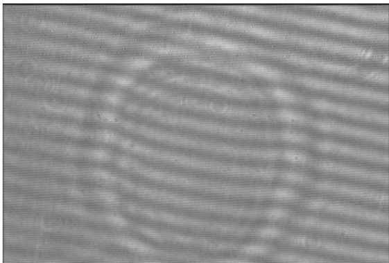
Fig. 4.11. Shock wave induced focusing a 6 ns laser pulse in air.
