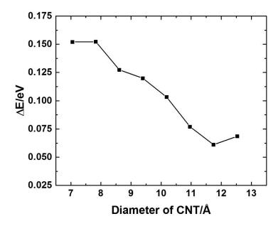
Figure 3-5. The difference in the potential energy between  $N_2$  and  $CO_2$  for different diameters of CNTs.
