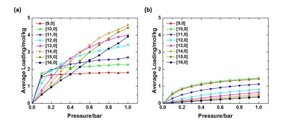
Figure 3-6. The isotherms of (a) CO<sub>2</sub> and (b) N<sub>2</sub> at 298K for different diameters of CNTs.
