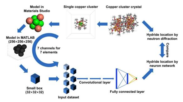
Figure 10-1. The process of generating input dataset and the sample architecture of 3D-CNN.
