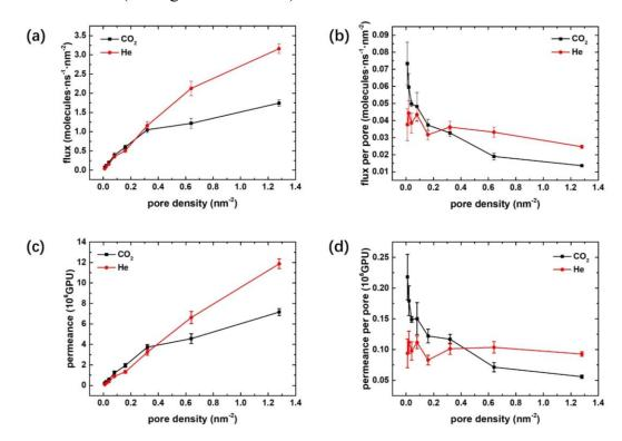
**Figure 4-3.** Initial flux and permeance vs pore density of graphene membranes for  $CO_2$  and He permeation: (a) flux per unit membrane area; (b) flux per pore; (c) permeance; (d) permeance per pore. Error bars from averaging over parallel simulations.
