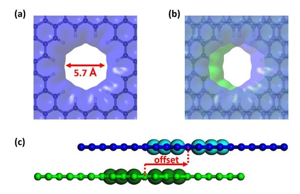
**Figure 5-1.** Construction of a porous bilayer graphene membrane: (a) the single-layer graphene with a relatively larger pore (5.7 Å in diameter) than the sizes of small gas molecules such as CO<sub>2</sub>; (b) the bilayer nanoporous graphene membrane from stacking two single-layer membranes from (a); (c) side view of the bilayer nanoporous graphene membrane. Isosurfaces of electron density are shown in (a) and (b) to define the pore shape; larger spheres in (c) indicate the pore rims.
