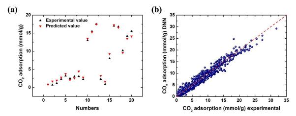
**Figure 8-2.** Results of predicted CO<sub>2</sub> uptakes. (a) Comparison between experiment and DNN-1 prediction for 20 pairs of CO<sub>2</sub> adsorption values. (b) The correlation between experiment and DNN-1 prediction for CO<sub>2</sub> uptakes by the leave-one-out method ( $R^2 = 0.96$ ).
