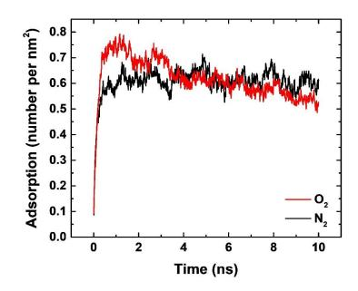
**Figure 6-4.** Adsorption amount on the feed site of the bilayer nanoporous graphene membrane (effective pore size at 3.45 Å) with time.
