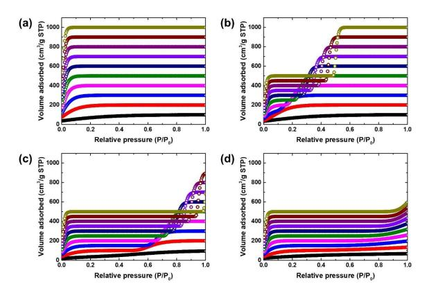
Figure S9-3. The N<sub>2</sub> adsorption isotherm examples from (a) group 1 ( $c_2 = -0.4 \sim 0.0$ ), (b) group 2 ( $c_2 = 0.1 \sim 0.5$ ), (c) group 3 ( $c_2 = 0.6 \sim 1.0$ ), and (d) group 4 ( $c_2 = 1.1 \sim 1.5$ ).
