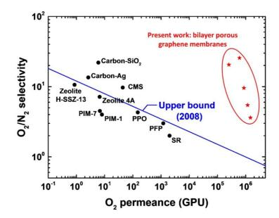
**Figure 6-9.** Comparison of bilayer porous graphene membranes to other membranes for  $O_2/N_2$  separation.<sup>8, 38</sup> The upper bound for polymer membranes is plotted with an assumed 1 µm-thick selective layer.<sup>38</sup> CMS: carbon molecular sieve; PPO: poly(phenylene oxide); PFP: perfluoropolymer; SR: silicone rubber.
