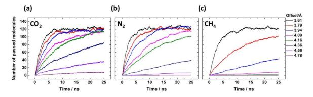
**Figure 5-2.** The number of gas molecules passing through the bilayer nanoporous graphene membrane vs. time for different offset values between the two single-layer graphene membranes: (a)  $CO_2$ , (b)  $N_2$  and (c)  $CH_4$ .
