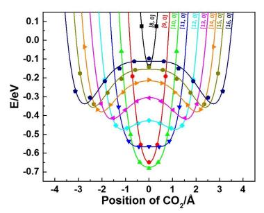
Figure 3-2. Potential energy surface of CO<sub>2</sub> in the CNTs calculated by the vdW-DF method.
