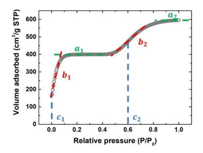
Figure S9-2. An N<sub>2</sub> adsorption isotherm at 77 K created by generation function ( $y = 400e^{-e^{-35(x-0)}} + 200e^{-e^{-10(x-0.6)}}$ ).
