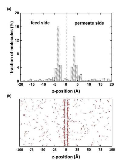
**Figure 4-4.**  $CO_2$  distribution along the z direction for a graphene membrane (at z=0) with the pore density of 1.28 nm<sup>-2</sup> after 25 ns MD simulation: (a) statistical distribution at the 25-ns time point (bin size: 1 Å); (b) snapshot of CO<sub>2</sub> distribution at the 25-ns time point.
