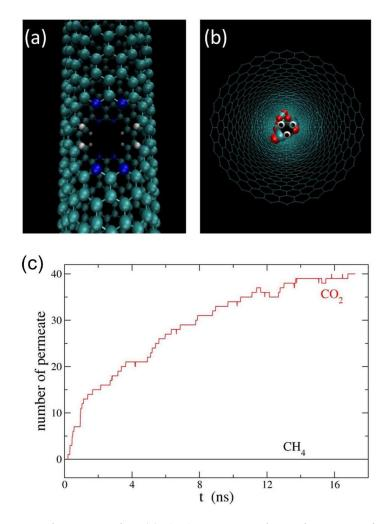
**Figure 1-6.** Porous carbon nanotube. (a) 4N4H pore on the carbon nanotube wall. (b) initial configuration of CMD simulation. (c) number of permeate molecules with time.<sup>36</sup>
