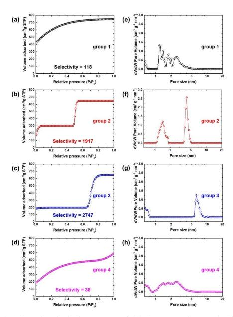
**Figure 9-4.** (a-d)  $N_2$  adsorption isotherm at 77 K and (e-h) the corresponding pore size distribution of the hypothetical porous carbon with the highest IAST CO<sub>2</sub>/N<sub>2</sub> selectivity in each group for 90 mol% N<sub>2</sub> and 10 mol% CO<sub>2</sub> at 298 K and total pressure of 1 bar.
