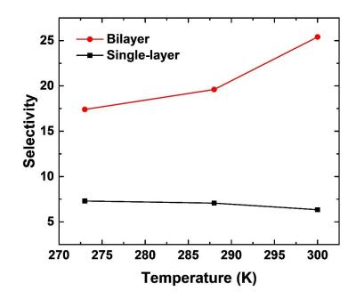
**Figure 6-8.** Change of  $O_2/N_2$  selectivity with temperature for single-layer and bilayer nanoporous graphene membranes.
