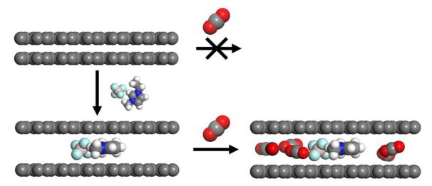
**Figure 7-1.** Schematic of the design of a composite material of graphene and an ionic liquid for gas adsorption. Ionic liquid is used to as a pillar to open up the space between graphene layers.
