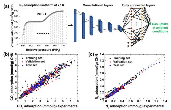
**Figure 9-1.** Results of predicted gas uptakes. (a) Architecture of the convolutional neural networks (CNN) used in this work: input, N<sub>2</sub> adsorption at 77 K; output, gas uptakes at ambient temperature
