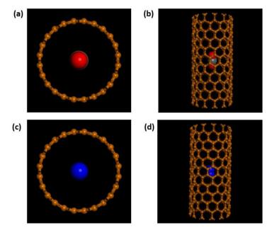
Figure 3-1. Structure of  $CO_2$  (a and b) and  $N_2$  (c and d) inside the carbon nanotube in our DFT modeling.
