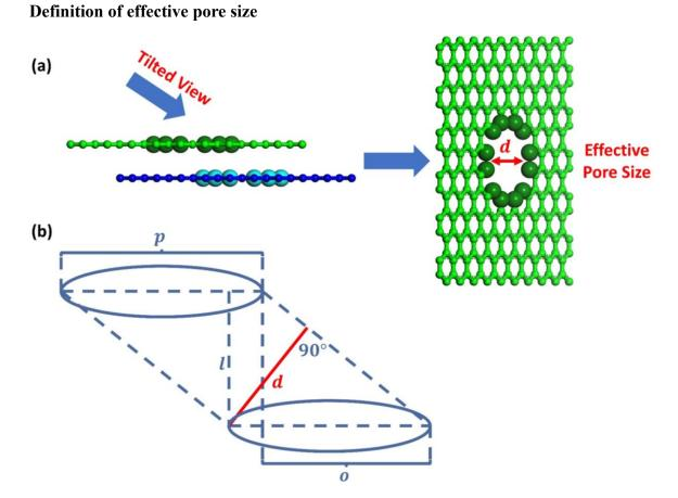
**Figure S5-1.** (a) Side view and tilted view of bilayer nanoporous graphene membrane; (b) Schematic of cross section of pore (5.7 Å).
