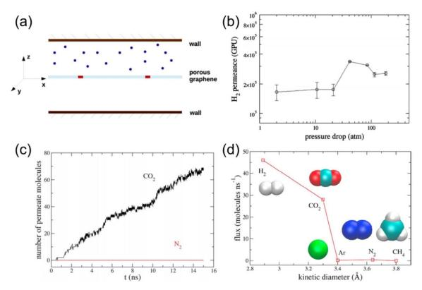
**Figure 1-4.** Examples of CMD simulations for gas separation. (a) The bi-chamber simulation model.<sup>31</sup> (b) H<sub>2</sub> permeance through the porous graphene at different pressure.<sup>31</sup> (c) CO<sub>2</sub> and N<sub>2</sub> permeation through nitrogen-functionalized nanopore (4N4H).<sup>32</sup> (d) Fluxes of several gas molecules through 4N4H nanoporous graphene by CMD simulations.<sup>33</sup>
