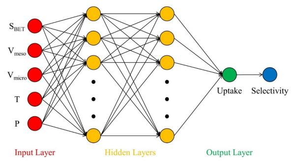
**Figure 8-1.** The deep neural networks (DNNs) used in the present work to predict gas uptake in porous carbons based on inputs from BET surface area ( $S_{BET}$ ), mesopore volume ( $V_{meso}$ ), micropore volume ( $V_{micro}$ ), temperature (T), and pressure (P).
