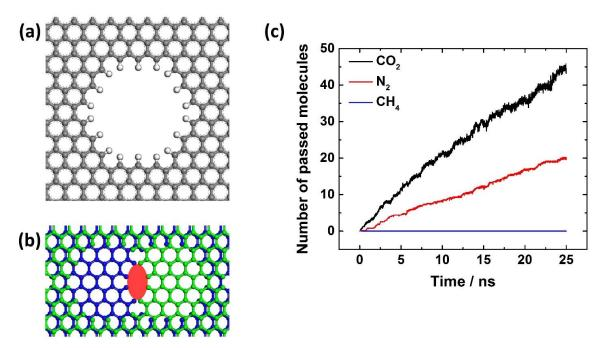
**Figure 5-6.** Bilayer membranes with pore size of 10.4 Å. (a) Structure of the graphene sheet with pore size of 10.4 Å; (b) the bilayer graphene membrane from two single-layer membranes from (a) at an offset of 9.3 Å (red oval represents the effective pore dimensions,  $\sim$ 3.6 Å in width); (c) permeation of CO<sub>2</sub>, N<sub>2</sub> and CH<sub>4</sub> with time through the bilayer graphene membrane in (b).
