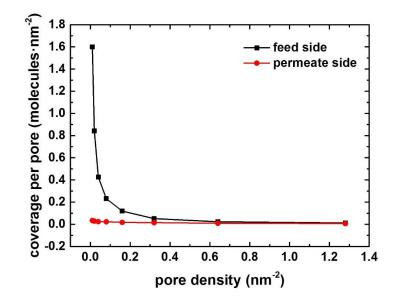
**Figure 4-9.** Coverage per pore of  $CO_2$  on feed side and permeate side of the graphene membrane of different pore densities.
