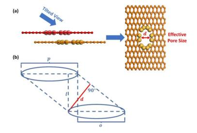
**Figure S6-1.** (a) Side view and tilted view of bilayer nanoporous graphene membrane; (b) Schematic of cross section of pore (5.7 Å).
