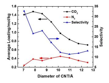
**Figure 3-8.** Gas uptake and  $CO_2/N_2$  selectivity from a mixture of  $CO_2$  (0.15 atm) and  $N_2$  (0.85 atm) at 298K for different diameters of CNTs.
