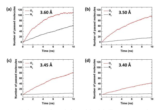
**Figure 6-2.** The numbers of gas molecules passed through the bilayer nanoporous graphene membranes with different effective pore sizes: (a) 3.60 Å; (b) 3.50 Å; (c) 3.45 Å; (d) 3.40 Å.
