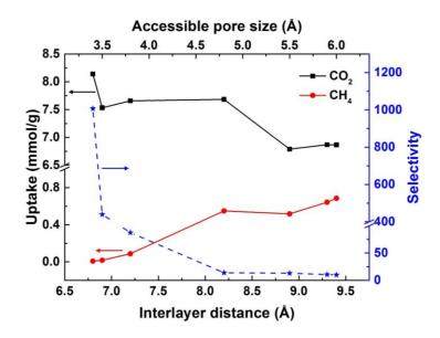
**Figure 7-6.** Uptakes of  $CO_2$  (black) and  $CH_4$  (red) by different GIL composites of 50/50  $CO_2/CH_4$  gas mixtures at 298K and 1 bar and corresponding selectivities (blue).
