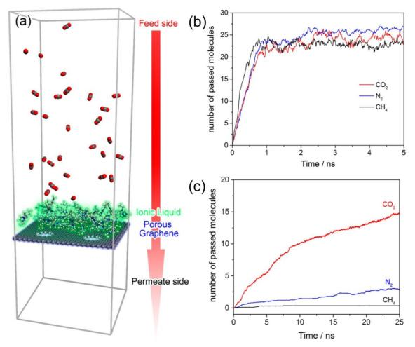
**Figure 1-5.** Porous graphene with one IL layer. (a) The simulation model of gas permeance through the porous graphene with one IL layer. Pure gas permeation through porous graphene membrane (b) without and (c) with IL layer.<sup>34</sup>
