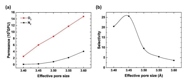
Figure 6-3.  $O_2$  and  $N_2$  permeances (a) and  $O_2/N_2$  permselectivity (b) of the bilayer nanoporous graphene membranes with different effective pore sizes.
