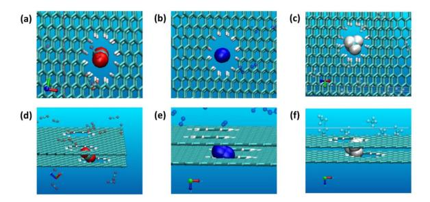
**Figure 5-5.** Snapshots of passing-through events of gas molecules: (a) and (d) CO<sub>2</sub>; (b) and (e) N<sub>2</sub>; (c) and (f) CH<sub>4</sub>. Upper pane, top view; lower panel, side view.
