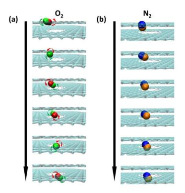
**Figure 6-5.** Snapshots of (a)  $O_2$  and (b)  $N_2$  passing through bilayer nanoporous graphene membrane with effective pore size of 3.45 Å.
