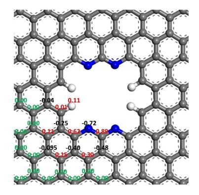
**Figure S4-1.** The 4N4H pore structure (carbon, grey; nitrogen, blue; hydrogen, white). The partial atomic charges used in our simulations are provided next to each atom. Due to the D2h symmetry of the pore structure, only the atoms in the lower left part are labelled with their atomic charges.
