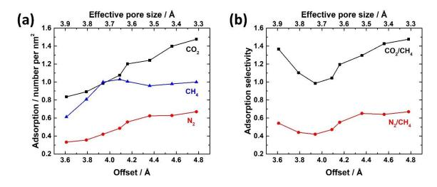
**Figure 5-4.** Adsorption amount of  $CO_2$ ,  $N_2$  and  $CH_4$  on the feed side (a) and adsorption selectivities of  $CO_2/CH_4$  and  $N_2/CH_4$  (b) as a function of the offset (bottom axis) or the effective pore size (top axis) in the bilayer nanoporous graphene membranes.
