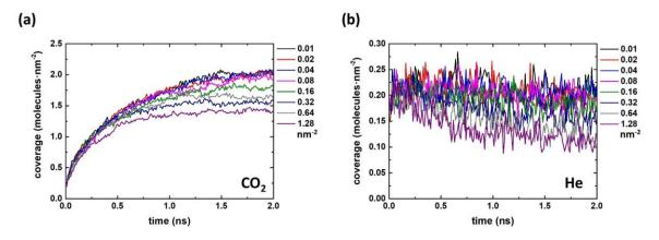
**Figure 4-5.** Coverage of the gas adsorbate vs time on the feed side of the graphene membranes of different pore densities: (a) CO<sub>2</sub>; (b) He.
