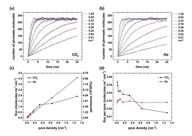
**Figure S4-2.** The number of gas molecules permeating through the nanoporous graphene membrane with time for different pore densities (from 0.01 to 1.28 nm<sup>-2</sup>): (a) CO<sub>2</sub>; (b) He; Dashed lines represent the exponential decay model fitting. Flux vs pore density of graphene membranes for CO<sub>2</sub> and He permeation: (c) flux and permeance per unit membrane area; (d) flux per pore.
