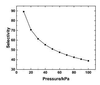
**Figure 3-9.** The IAST-predicted  $CO_2/N_2$  selectivity as a function of total pressure for a mixture of  $CO_2$  and  $N_2$  in 0.15/0.85 molar ratio in CNT [9, 0].
