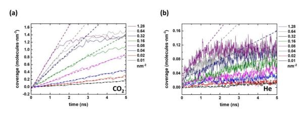
**Figure 4-6.** Coverage of the adsorbate vs time on the permeate side of the graphene membrane of different pore densities: (a) CO<sub>2</sub>; (b) He.
