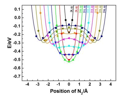
Figure 3-3. Potential energy surface of N<sub>2</sub> in the CNTs calculated by the vdW-DF method.
