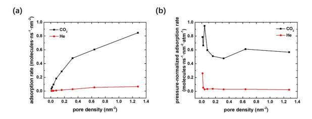
**Figure 4-7.** (a) Adsorption rate and (b) pressure-normalized adsorption rate on the permeate side vs the pore density for  $CO_2$  and He.
