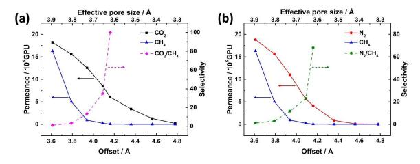
**Figure 5-3.** Permeance (left axis) and selectivity (right axis) as a function of the offset (bottom axis) or the effective pore size (top axis) in the bilayer nanoporous graphene membranes: (a)  $CO_2$  vs.  $CH_4$ ; (b)  $N_2$  vs.  $CH_4$ .
