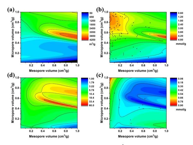
**Figure 8-6.** The 2D contour maps of (a) BET surface areas  $(m^2/g)$ , (b) CO<sub>2</sub> and (c) N<sub>2</sub> adsorption capacities (mmol/g), and (d) CO<sub>2</sub>/N<sub>2</sub> selectivity for 2500 hypothetical porous carbons at 298 K and 1 bar. The black dots in (b) and (c) represent the experimental data points at the same condition.
