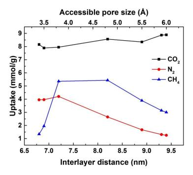
**Figure 7-4.** Uptakes of pure gas molecules ( $CO_2$  – black,  $N_2$  – red,  $CH_4$  – blue) at 298K and 1 bar by different GIL composites.
