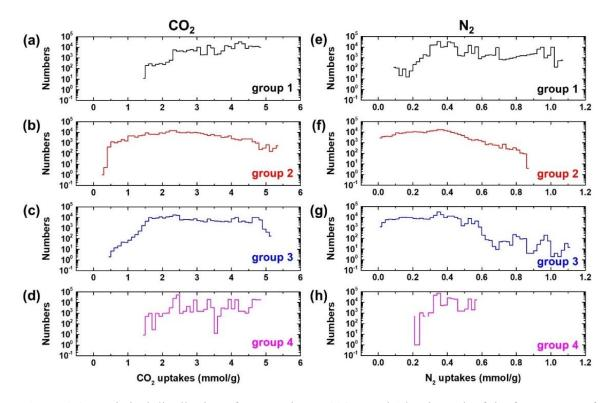
**Figure 9-2.** Statistical distribution of gas uptakes at 298 K and 1 bar in each of the four groups of hypothetical porous carbons: (a-d) CO<sub>2</sub>; (e-h) N<sub>2</sub>.
