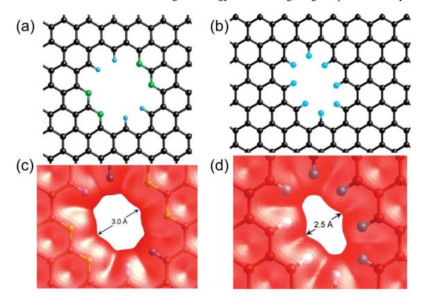
**Figure 1-3.** Two types of nanopores in graphene sheet. (a) all-hydrogen saturated pore; (b) nitrogen-functionalized pore. (c) and (d) are their electron density isosurface.<sup>29</sup>
