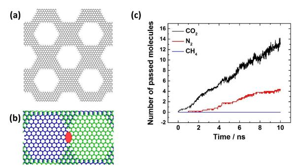
**Figure 5-7.** Bilayer membranes with pore size of 25.2 Å. (a) Structure of the graphene sheet with pore size of 25.2 Å; (b) the bilayer graphene membrane from two single-layer membranes from (a) at an offset of 24.0 Å (red oval represents the effective pore dimensions;  $\sim$ 3.6 Å in width); (c) permeation of CO<sub>2</sub>, N<sub>2</sub> and CH<sub>4</sub> with time through the bilayer graphene membrane in (b).
