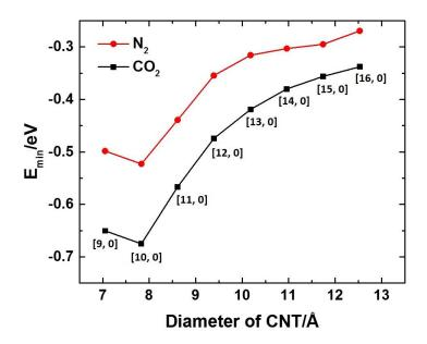
Figure 3-4. The minimum values of potential energy for different diameters of CNTs.
