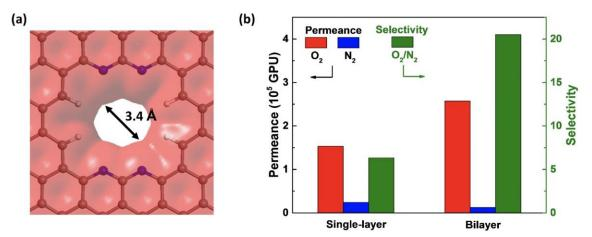
**Figure 6-6.** Comparison between single-layer and bilayer graphene membrane. (a) A single-layer porous graphene membrane with a pore of an elliptic shape and an average pore size of 3.4 Å. (b) Comparison of  $O_2$  and  $N_2$  permeances as well as  $O_2/N_2$  selectivity between a single-layer graphene with a pore size of 3.4 Å and the bilayer graphene membrane with an effective pore size of 3.4 Å.
