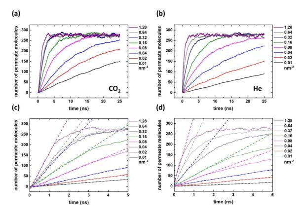
**Figure 4-2.** The number of gas molecules permeating through the nanoporous graphene membrane with time for different pore densities (from 0.01 to  $1.28 \text{ nm}^{-2}$ ): (a) CO<sub>2</sub> in 25 ns; (b) He in 25 ns; (c) CO<sub>2</sub> in 5 ns; (d) He in 5 ns. Dashed lines in (c) and (d) denote the permeation rates used to compute the initial fluxes.
