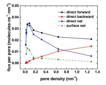
**Figure S4-3.** The forward, backward, and net direct fluxes, in comparison with the net surface flux of He, across graphene membranes of different pore densities.
