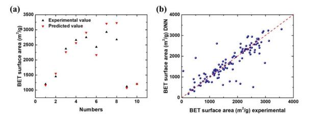
DNN-3 provides a reasonably good model to correlate V<sub>micro</sub> and V<sub>meso</sub> to S<sub>BET</sub>.
