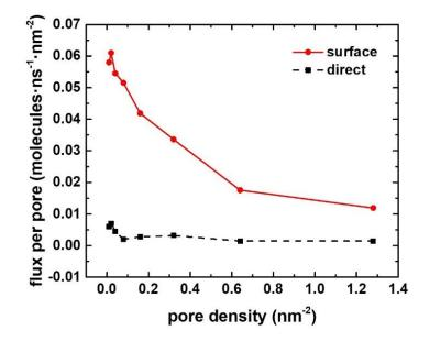
**Figure 4-8.** The surface flux and the direct flux of CO<sub>2</sub>, across graphene membranes of different pore densities. The values are from the trajectory analysis of all gas molecules during the initial 1 ns.
