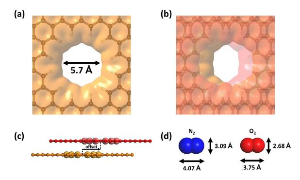
**Figure 6-1.** Construction of a porous bilayer graphene membrane: (a) Single-layer graphene pore; (b) bilayer nanoporous graphene membrane; (c) side view of the bilayer nanoporous graphene membrane with an offset of the two pore centers (the larger spheres indicate the pore rims); (d) molecular sizes of nitrogen and oxygen. In (a) and (b), the pore shapes and sizes are estimated by the isosurfaces of electron density at 0.0004  $e/a_0^3$ .
