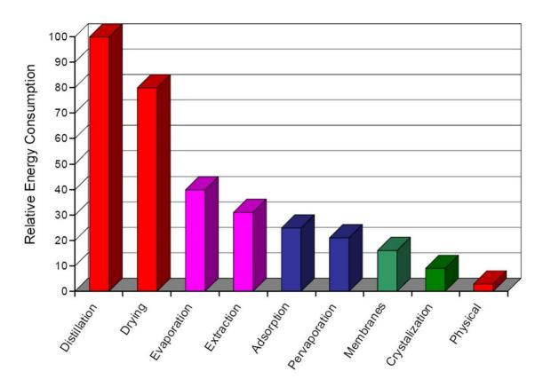
Figure 1-1. Relative energy use by various separation technologies.<sup>2</sup>
