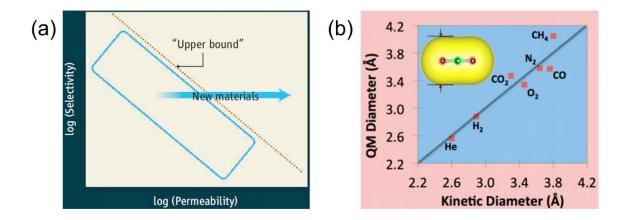
**Figure 1-2.** Robeson upper bound and molecular diameters. (a) The trade-off between selectivity and permeability called Robeson upper bound.<sup>22</sup> (b) Comparation between the QM diameters with the experimental kinetic diameters.<sup>24</sup>
