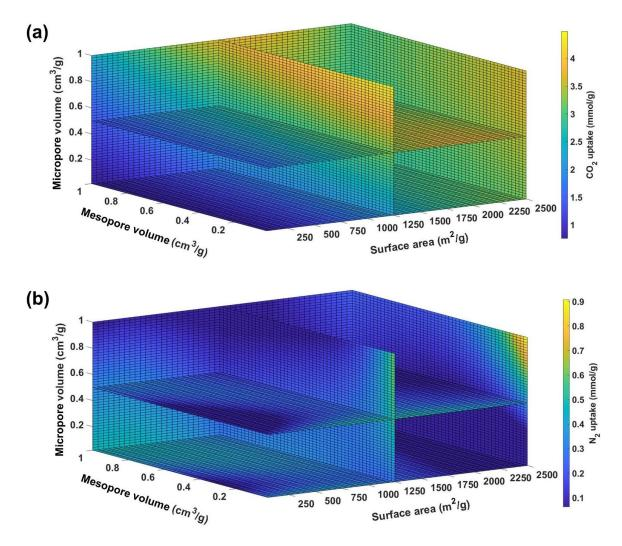
**Figure 8-4.** The 3D contour maps of (a)  $CO_2$  and (b)  $N_2$  pure-gas adsorption capacities at 298 K and 1 bar in 125000 hypothetical porous carbons predicted from DNN-1 and DNN-2, respectively.
