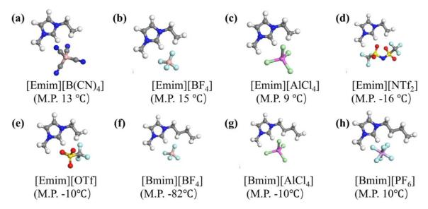
Figure 7-3. Eight room-temperature ionic liquids in our work and their melting points.
