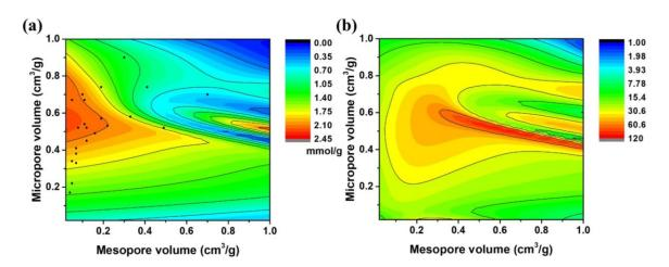
**Figure 8-7.** The 2D contour maps of (a)  $CO_2$  adsorption capacity at 298K and 0.15 bar, and (b)  $CO_2/N_2$  selectivity for 0.15 bar  $CO_2$  vs 0.85 bar  $N_2$  at 298 K. The black dots in (a) represent the experimental data points.
