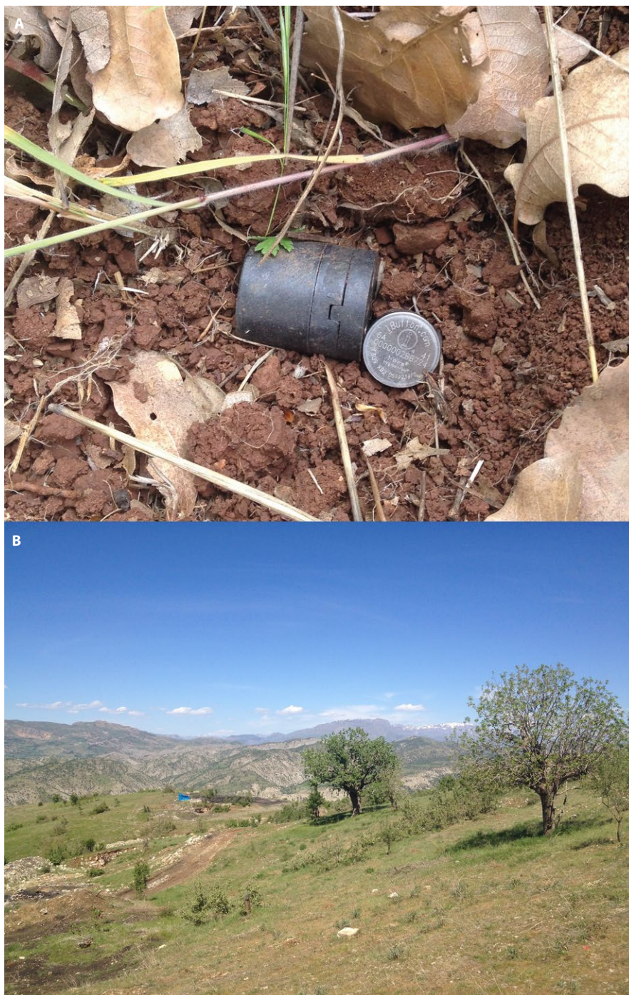
FIGURE 3. (A) Placement of iButton Hygrochrons and Thermochrons (within black iButton capsules) into soils 5 cm below the surface near Cicer plants. (B) Typical wild Cicer habitat in southeastern Turkey (from the Cudi habitat in von Wettberg et al., 2018).
