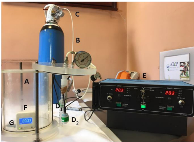
Fig. 3. Image illustrating the hypoxia-inducing chamber and gas apparatus. A plexiglass cylinder (A) was used as a chamber to house the Drosophila during treatment. Nitrogen gas was introduced into the system by a tube (B) connected to a nitrogen tank (C). Two oxygen probes (D 1 and D 2 ) were connected to an external monitor (E). A third oxygen probe was in the CUBO 2 device (F). Environmental conditions inside the chamber during experiments were monitored using a MSR145 data logger (G).
