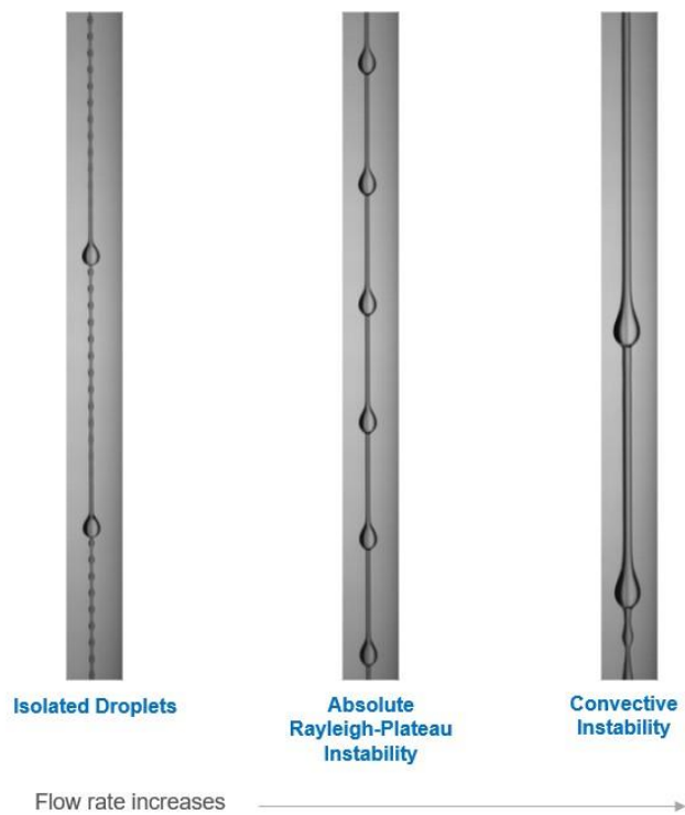
Figure 1.2: Silicone oil v50 flowing on a monofilament with 0.2 mm thickness. The mass flow rate increases from 0.006 g/s to 0.02 g/s to 0.1 g/s from left to right.
