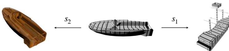
Figure 7.2: Shape vs. texture task. s_1 represents the cosine similarity between the query object x and a different object with the same texture x_t . s_2 represents the cosine similarity between the query object x and the same object with a different texture x_s . We call the decision texture-biased if s_1 > s_2 and shape-biased otherwise.
