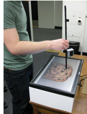
Figure 2: The display used in the experiment. Participants used the black rod to indicate the orientation at which the highlighted region extended into the object.
