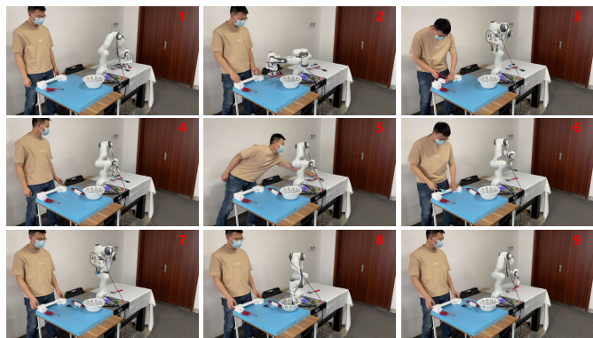
Fig. 8. The Human operator and robotic manipulator work in a shared workspace. Fig. 8.5-Fig. 8.9 demonstrate that, when the human is assistive, the robot can determine the current task progress and continue on subsequent tasks. The experiment video is available at https://youtu.be/jKXuOJu1MsA .
