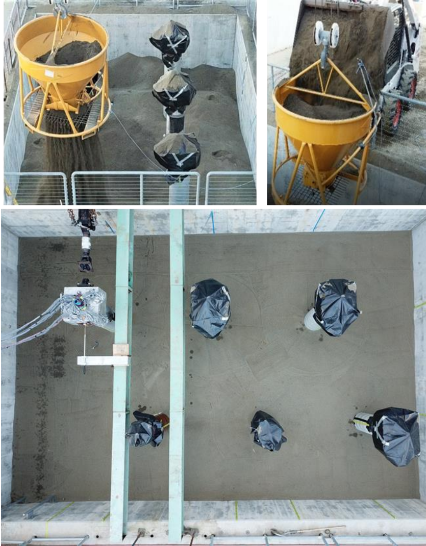
Figure 3-20 Sand pluviation process
