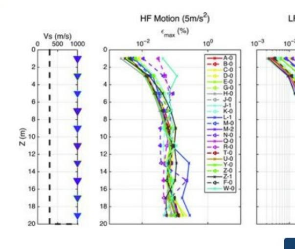
Peak shear-strain profiles reached at each depth by each team for the HF and LF PGA level (5 m/s<sup>2</sup>), for profile 1 and for rigid substratum conditions.
