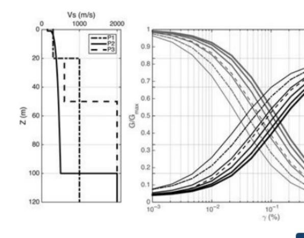
V<sub>S</sub> profiles, G/G<sub>max</sub>, and damping curves for the three idealized profiles.
