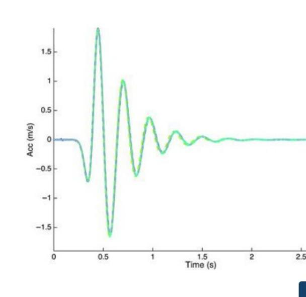
Comparison of the acceleration at the surface of P1 profile, for the pulse-like inp computation and for the elastic substratum case.
