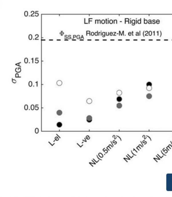
Standard deviation (in log unit) of PGA for profiles 1, 2, and 3, for the five differe linear-viscoelastic, NL with input motion scaled to the lowest).
