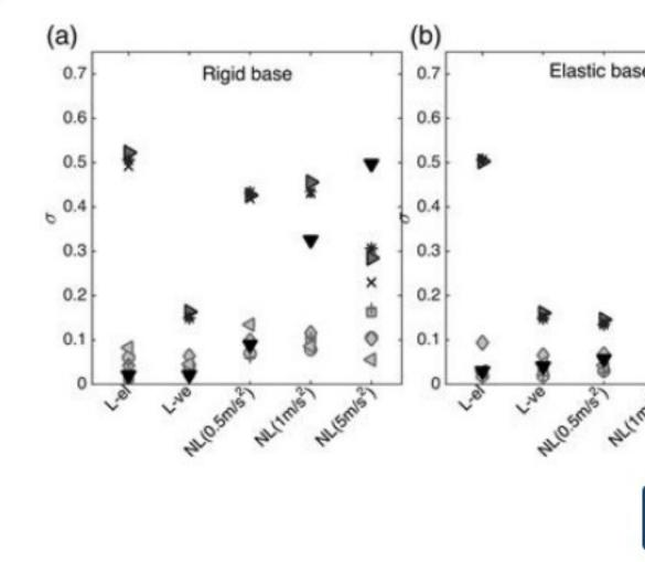
Standard deviation (in log unit) of the different intensity parameters for the P1 computational cases: linear-elastic, linear-viscoelastic, NL with input motion (1 m/s<sup>2</sup>), and highest (5 m/s<sup>2</sup>) PGA, for the LF content motion. (a) The results elastic substratum.
