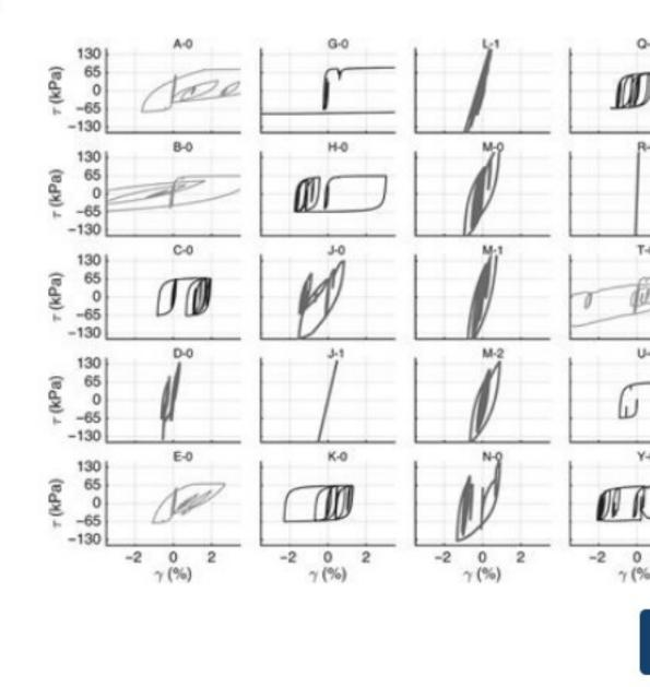
Stress-strain curves at the bottom of the P1 profile for the rigid substratum cas the highest PGA [5 m/s<sup>2</sup>]). The thicker curves are for code/team couples that e 65 kPa, whereas the thin curves represent the code/team couples that use 65 k using damping control and the darker curves the others.
