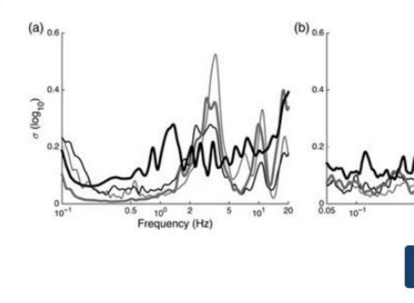
Standard deviation (in log unit) of the (a) transfer function and (b) response specused.
