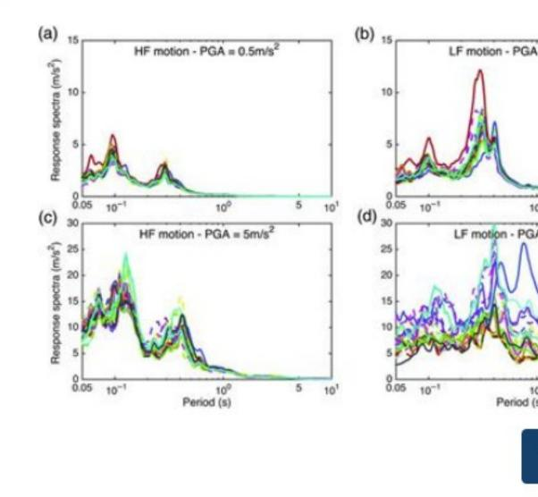
Comparison of the acceleration pseudoresponse spectra at the ground surface, to input motion (a) scaled to 0.5 m/s<sup>2</sup> and (c) scaled at 5 m/s<sup>2</sup>, and using the LF inp (d) scaled at 5 m/s<sup>2</sup>.
