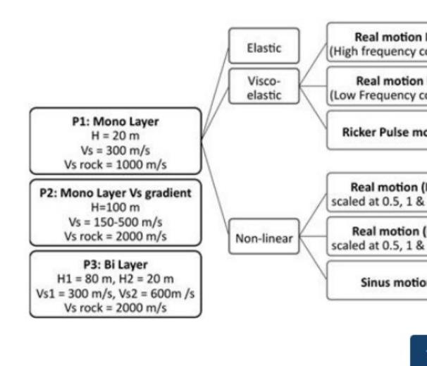
The three simple idealized profile cases studied here (P1–P3), for the elastic and elastic soil-bedrock base, using a Ricker pulse and three accelerations of differer frequency contents.
