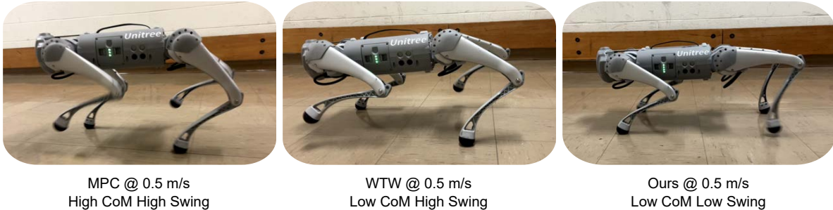
Figure 8.5: Three policies walking at 0.5 m/s. Built-in MPC and walk-these-ways (WTW) [130] swing the legs to a redundant height, while our policy only makes necessary lifting of the leg. This demonstrates the energy-efficiency of our policy.
