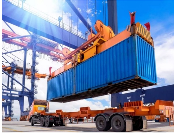
Figure 4.1: A truck with skeleton chassis receiving two 20 ft. containers at a port.
