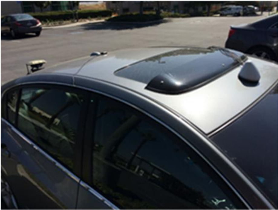
Figure 25. Three Receivers Were Installed on Test Vehicle for Measuring Positioning Accuracy
