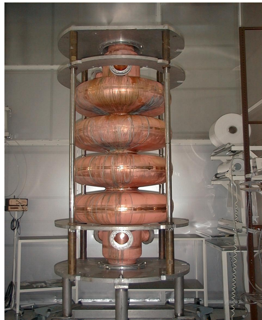
Figure 7: Prototype cavity optimized for \beta = 0.7 .
