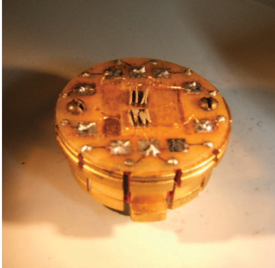
Figure II.12: Photograph of the PPMS sample puck with two samples mounted for a four-wire resistivity measurement.
