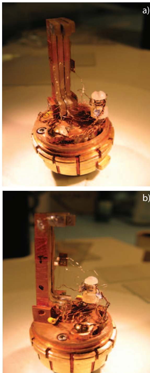
Figure II.13: Photograph of the modified PPMS puck used for thermopower measurements. a) Side view. b) Front view.
