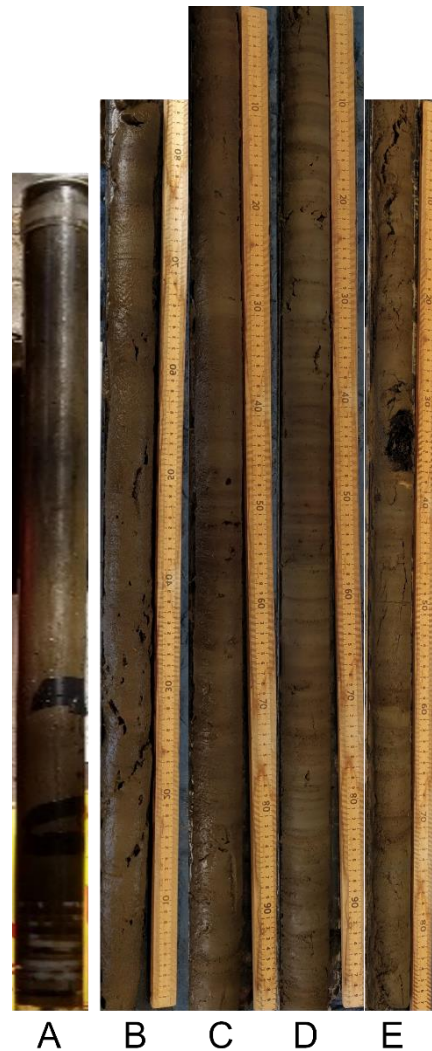
Figure 3-3 Core stratigraphy images of KLGC 19-1 and KLRC 19-2. A) KLGC19-1 (0 – 87.5 cm), B-E) KLRC19-2 Drive(D) 1 (87.5 – 175 cm), D2 (175 – 275 cm), D3 (275 – 375 cm), and D4 (375 – 462 cm).
