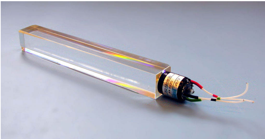
Figure 5.1: CMS Electromagnetic Calorimeter Lead Tungstate Crystal [4].
