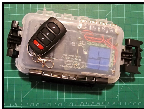
Figure 6: A) Simple and B) radio-frequency controllers for electronic modules. The devices contain four on/off switches which control and distribute the electric supply for each of the four USB outputs. They require a standard 5v USB power source.
