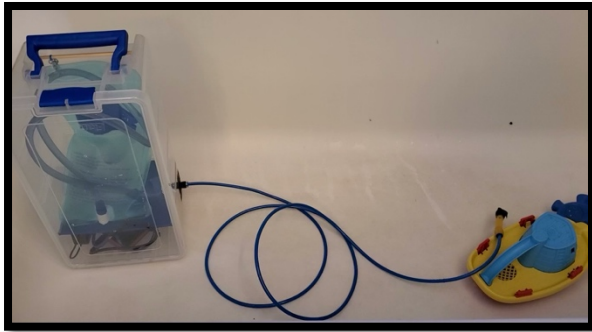
Figure 9: Water pump module. (Left) The plastic housing contains the water bladder, water pump, pulse generator module, and power supply. (Middle) A non-compressible air brake tubing transmits the water to a segment of (Right) latex tubing. A child's bath toy is provided for scale.
