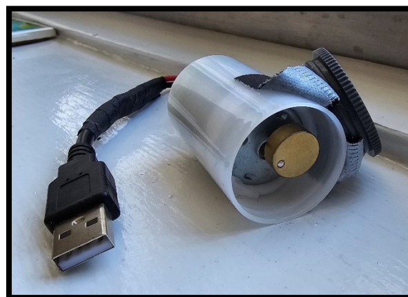
Figure 8: Electronic module vibrating motor to simulate seizures. A) External view. B) View demonstrating the internal vibrating motor.
