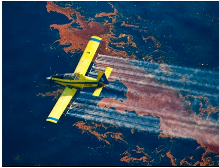
Figure 2.2: Aerial spraying of chemical dispersant, a method referred to as "carpet bombing". Image courtesy of Stephen Lehmann, USCG.
