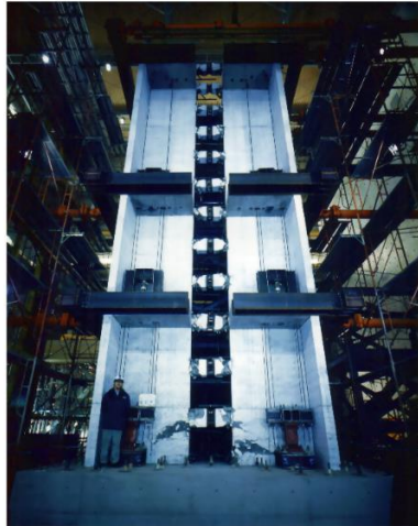
a. Elevation View of Deformed Coupled Wall
