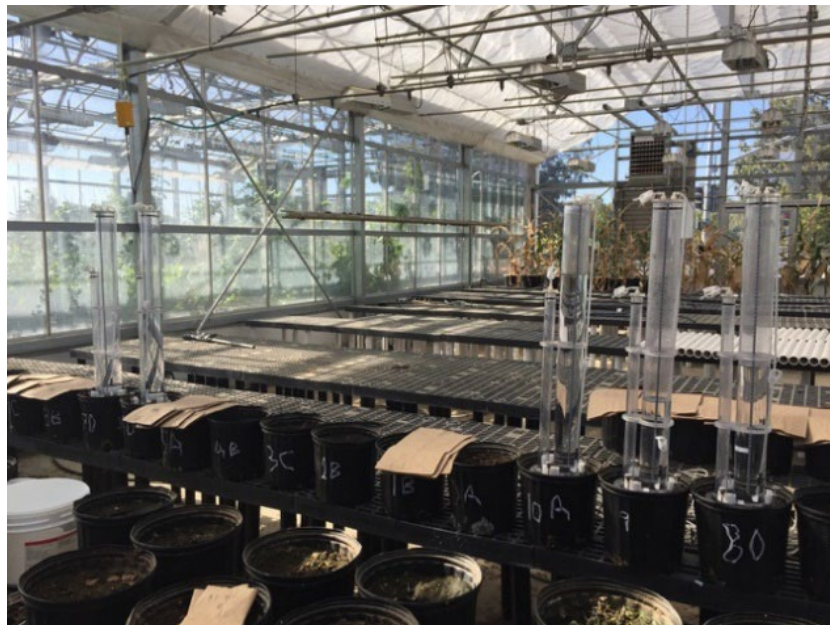
Figure 3-6. Showing Wooding Infiltrometer Placed on Top of Different Treatment Pots at the End of the Strawberry Experiment in a UC Davis Core Facility Greenhouse.
