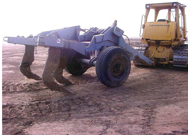
Figure 2-11. The Deep Ripper That Does Not Turn the Soil over Used for Improving Drainage in Clay Soils.
