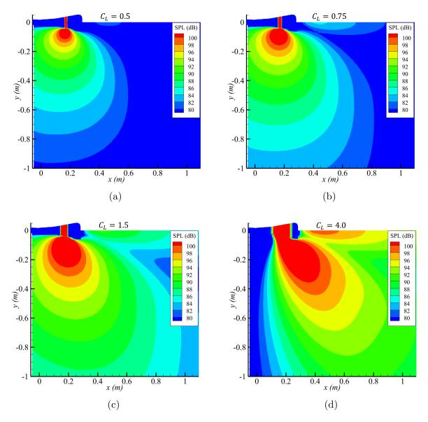
Figure 5.5: Sound pressure levels generated by wavepackets of different length scales, all other parameters equal.
