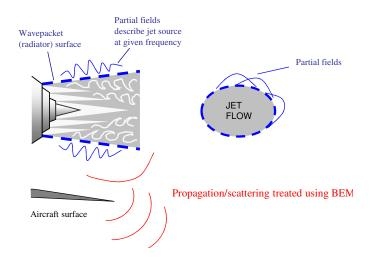
Figure 2.6: Basic elements of surface-based modeling of the jet noise source.
