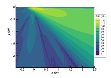
Figure A.6: Sound pressure levels generated from the long cylinder using a wavepacket of length scale  $L = 5\hat{D}$  along the vertical half-plane. The cylinder is visible near y = 0, spanning from x = -0.4 m to x = 2.5 m.
