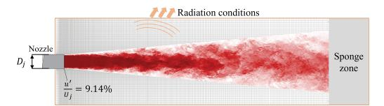
Figure 3.1: Visualization of the single-stream jet over the numerical grid, with its boundary conditions. The jet contour plots instantaneous axial velocity from 0 (white) to  $U_j$  (red).
