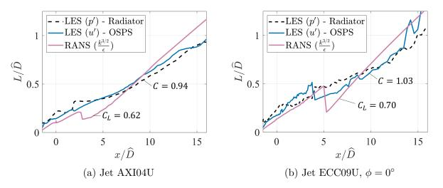
Figure 4.34: Fitting of  $L_u$  on the OSPS and RANS-based length scales to the  $L_p$  distribution on the radiator surface.
