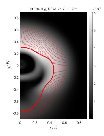
Figure 4.8: Detection of the outer surface of peak Reynolds stress (OSPS) at  $x/\hat{D} = 1.467$  for jet ECC09U. Contours indicate the distribution of Reynolds stress on this cross-stream plane. Thin red lines: rays along the mean velocity gradient. Thick red line: OSPS
