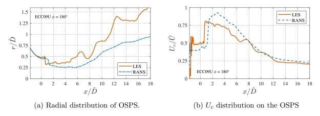
Figure 4.13: RANS and LES results regarding the OSPS of jet ECC09U on  $\phi = 180^{\circ}$ .
