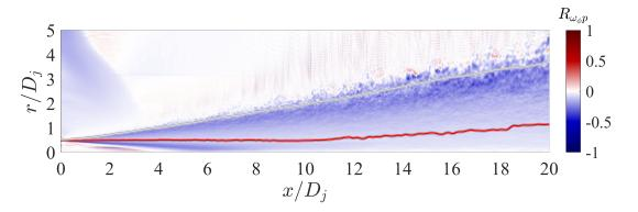
Figure B.3: Distribution of the normalized correlation between  $\omega'_{\phi}$  and p',  $R_{\omega_{\phi}p}$ . Red line: SPS. White line: radiator surface.
