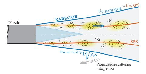
Figure 3.9: Representation of wavepacket model for the single-stream jet.
