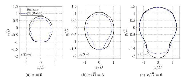
Figure 4.21: Comparison of radiator surface with surface based on the mean vorticity criterion of Eq. 4.4 using the RANS flow fields on three cross-sectional planes of jet ECC09U.
