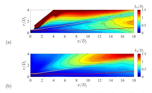
Figure 3.16: Isocontours of normalized length scales (a)  $L_u/D_j$  and (b)  $L_p/D_j$ . Red line: SPS. White line: radiator surface.
