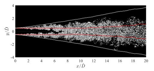
Figure 3.13: Representation of swirling strength at the value  $\lambda_{ci} = U_j/D_j$ . White double line: radiator surface. Red line: SPS.
