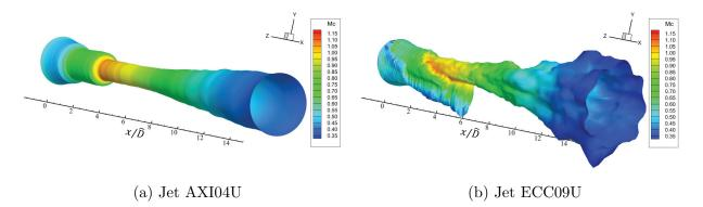
Figure 4.10: LES-based OSPS with contours of convective Mach number  $M_c$ .
