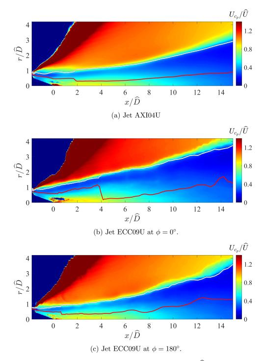
Figure 4.14: Distribution of normalized convective velocity  $U_{c_p}/\hat{U}$  as determined by spacetime correlations based on p' on the meridional planes of jets AXI04U and ECC09U. White lines: radiator surface; red lines: OSPS based on LES.
