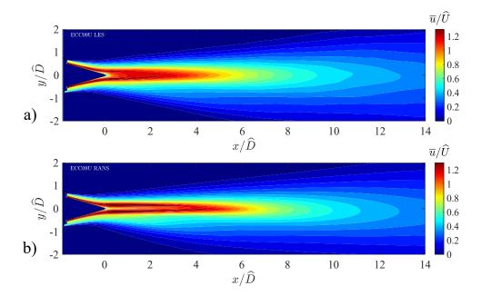
Figure 4.5: Isocontours of normalized normalized mean axial velocity  $\overline{u}/\hat{U}$  on the symmetry plane of jet ECC09U. a) LES and b) RANS.
