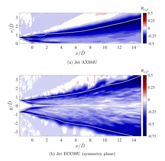
Figure 4.28: Distribution of normalized correlation between  $\omega'_{\phi}$  and p',  $R_{\omega_{\phi}p}$ . White lines: radiator surface.
