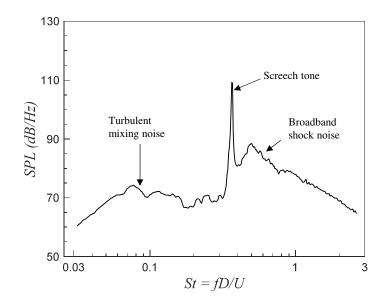
Figure 2.1: Far field noise spectrum of an overexpanded jet at a Mach number of 1.5. The microphone is at 150° to the downstream jet axis. Data from Seiner [97].
