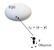
Figure A.1: Sketch of BEM surface and observer references.
