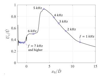
Figure 5.8: Convective velocity distribution  $U_c$  (solid line) and values assigned to the modeled wavepackets (circles) for  $C_f = 0.6$ .
