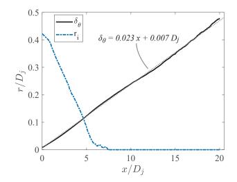
Figure 3.5: Axial distributions of momentum thickness  $\delta_{\theta}/D_j$  (solid black line) and inner edge of shear layer  $r_i/D_j$  (dashed blue line). Dotted line indicates linear fit.
