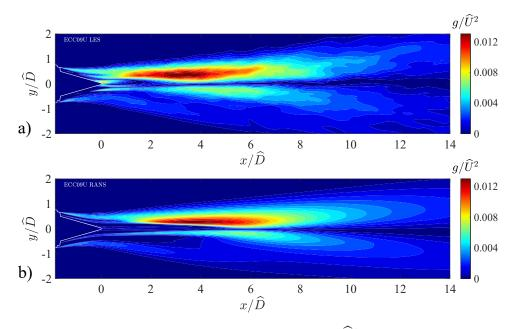
Figure 4.7: Isocontours of normalized Reynolds stress  $g/\hat{U}^2$  on the symmetry plane of jet ECC09U. a) LES and b) RANS.
