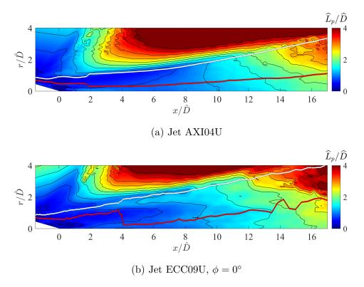
Figure 4.33: Isocontours of normalized moving-frame length scales based on pressure fluctuation,  $\hat{L}_p/\hat{D}$ . Red line: OSPS. White line: radiator surface.
