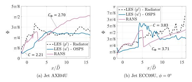
Figure 4.38: Fitting of  $\Phi_u$  on the OSPS and RANS-based azimuthal scales to the  $\Phi_p$  distribution on the radiator surface.
