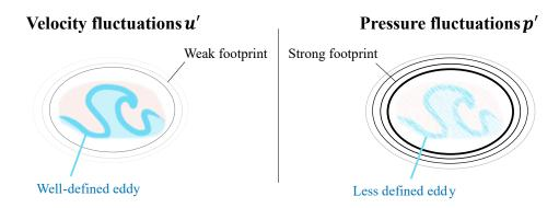
Figure 3.17: Simplified sketch of an eddy representation through velocity and pressure fluctuations.
