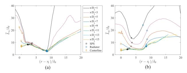
Figure 3.22: Plots of normalized moving-frame length scales  $\hat{L}/\delta_{\theta}$  versus similarity coordinate  $(r - r_i)/\delta_{\theta}$ , (a) based on axial velocity; (b) based on pressure. Legend applies to both subfigures.
