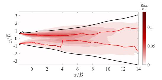
Figure 4.23: Distribution of the root mean square of pressure fluctuation on the symmetry plane of jet ECC09U. Black line: radiator surface. Red line: OSPS.
