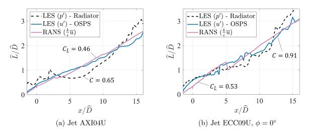
Figure 4.35: Fitting of  $\hat{L}_u$  on the OSPS and RANS-based length scales to the  $\hat{L}_p$  distribution on the radiator surface.
