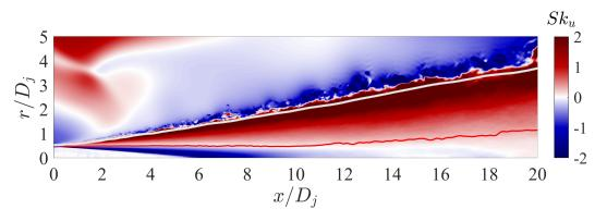
Figure B.2: Distribution of the skewness of the fluctuation of axial velocity,  $Sk_u$ , of the single-stream jet. Red line: SPS. Black double line: radiator surface.
