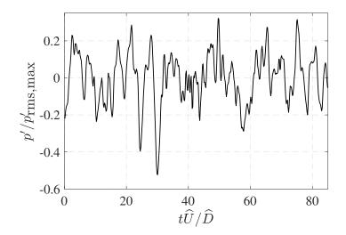
Figure 4.25: Pressure time history on the radiator surface of jet AXI04U at  $x/\hat{D} = 6$  and  $\phi = 0^{\circ}$ .
