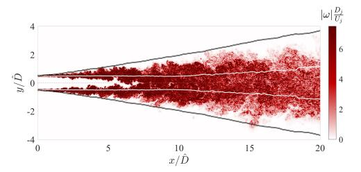
Figure 3.12: Contour of instantaneous vorticity norm along a longitudinal plane. Black double line: radiator surface. White line: SPS.
