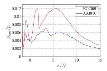
Figure 4.22: Distribution of  $p'_{\rm rms}$ , normalized by the ambient pressure  $p_{\infty}$ , on the radiator surfaces of jets AXI04U and ECC09U at  $\phi = 0^{\circ}$ .
