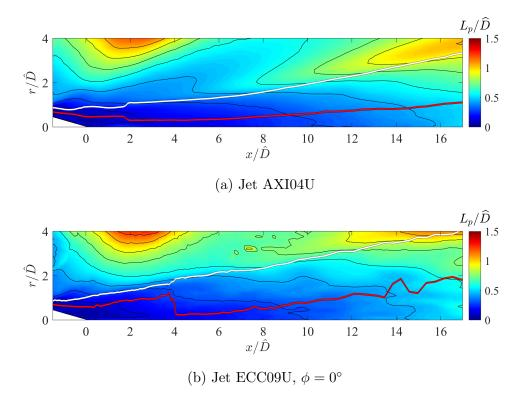
Figure 4.31: Isocontours of normalized fixed-frame length scales based on pressure fluctuation,  $L_p/\hat{D}$ . Red line: OSPS. White line: radiator surface.
