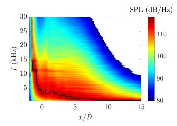
Figure 5.9: Pressure spectra along the radiator surface. The black line denotes the maximum frequency at each axial location.
