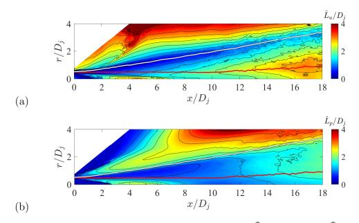
Figure 3.20: Isocontours of normalized length scales (a)  $\hat{L}_u/D_j$  and (b)  $\hat{L}_p/D_j$ . Red line: SPS. White line: radiator surface.
