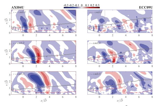
Figure 4.29: Contours of  $R_{up}$  with reference point  $(x_0, r_0) = (2, 0.3)\widehat{D}$  for jets AXI04U (left column) and ECC09U (right column) at azimuthal angle  $\phi = 0^{\circ}$ . Time separations:  $\tau = -1.92\widehat{D}/\widehat{U}$  (top row),  $\tau = 0$  (middle row), and  $\tau = 1.92\widehat{D}/\widehat{U}$  (bottom row). Red line: SPS. White line: radiator surface. Black dashed vertical line: positions for a downstream convection at velocity  $0.6\widehat{U}$ .
