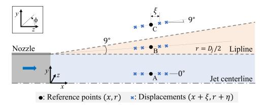
Figure 3.2: Examples of stencils used in the determination of length scales. Reference points are located (A) between centerline and lipline, (B) between lipline and 9° edge, and (C) outside 9° edge.
