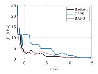
Figure 5.3: Peak frequencies of the pressure autospectra on the OSPS and radiator surface of jet AXI04U. RANS-based frequencies are adjusted by  $C_f = 0.3$ .
