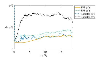
Figure 3.26: Axial distribution of azimuthal scales  $\Phi$  on the relevant surfaces. Orange solid line:  $\Phi_u$  on SPS. Blue dashed line:  $\Phi_u$  on the radiator surface. Green dotted line:  $\Phi_p$  on the SPS. Black line dash-dot:  $\Phi_p$  on the radiator surface.
