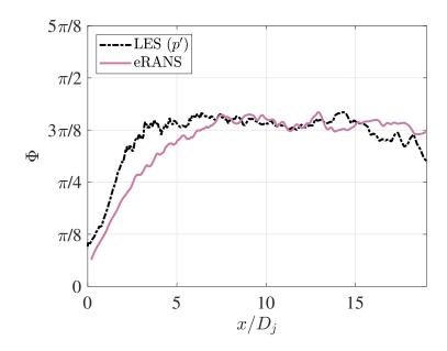
Figure 3.32: Fitting of eRANS-based azimuthal scales on the radiator surface with  $C_{\Phi} = 2.60$ .
