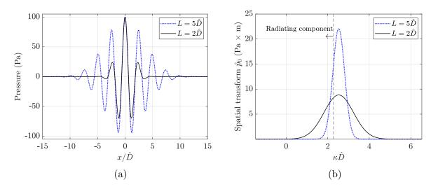
Figure A.2: Examples of wavepacket ansatzes for  $U_c = 0.9a_{\infty}$  and length scales of 2 and 5  $\hat{D}$ . (a) Real part of the axial distribution  $p_0(x)$ , and (b) Spatial Fourier transform  $\hat{p}_0(\kappa)$
