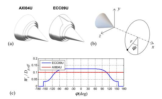
Figure 4.1: Characteristics of three-stream nozzles. (a) Exit geometry of nozzles; (b) coordinate system; (c) azimuthal variation of the tertiary annulus width.
