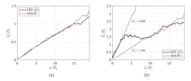
Figure 3.31: Fitting of eRANS-based length scales on the radiator surface. (a) Fixed-frame scale with  $C_L = 0.76$ ; (b) moving-frame scale with  $C_L = 5.65$  and  $C_L = 1.65$  for the initial region and for the region past the potential core, respectively.
