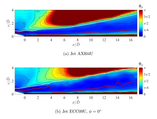
Figure 4.37: Isocontours of azimuthal scales based on pressure fluctuation,  $\Phi_p$ . Red line: OSPS. White line: radiator surface.
