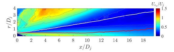
Figure 3.8: Isocontours of normalized convective velocity  $U_{c_u}/U_j$  on a meridional plane. Red line: SPS. White line: radiator surface.
