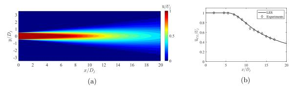
Figure 3.4: Distribution of normalized mean axial velocity. (a) Isocontours on a symmetry plane; (b) axial distribution on jet centerline compared to experiments by Lau *et al.* [56].
