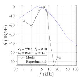
Figure 5.6: Comparison of scaled experimental and modeled autospectra using a length scale coefficient of  $C_L = 4.0$ .
