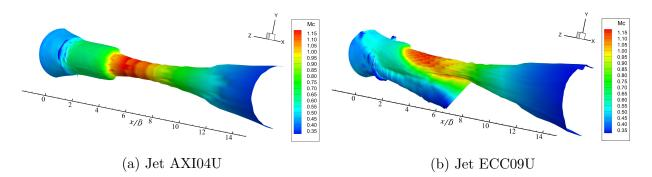
Figure 4.9: RANS-based OSPS with contours of convective Mach number  $M_c$ .
