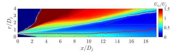
Figure 3.7: Isocontours of normalized convective velocity  $U_{c_p}/U_j$  on a meridional plane. Red line: SPS. White line: radiator surface.
