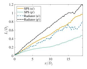
Figure 3.18: Axial distribution of the correlation scales L on the relevant surfaces. Orange solid line:  $L_u$  on SPS. Blue dashed line:  $L_u$  on the radiator surface. Green dotted line:  $L_p$  on SPS. Black line dash-dot:  $L_p$  on the radiator surface.
