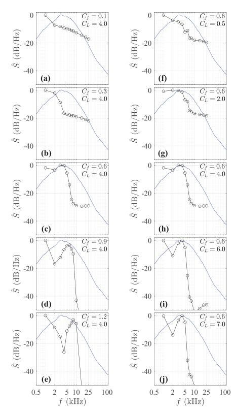
Figure 5.7: Changes in modeled autospectrum generated by changing  $C_f$  (left column) or  $C_L$  (right column) around point  $C_f = 0.6$  and  $C_L = 4.0$ . Wavepacket amplitude is  $\mathcal{A} = 1$  for all cases.
