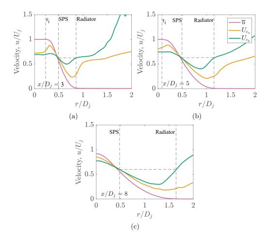
Figure 3.10: Radial distributions of  $\overline{u}$ ,  $U_{c_u}$ , and  $U_{c_p}$  at (a)  $x/D_j=3$ , (b)  $x/D_j=5$ , and (c)  $x/D_j=8$ . Legend is the same for all plots.
