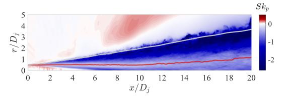
Figure B.1: Distribution of the skewness of the pressure fluctuation,  $Sk_p$ , of the single-stream jet. Red line: SPS. White line: radiator surface.
