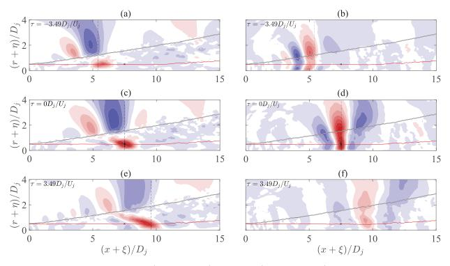
Figure 3.15: Contours of  $R_{uu}$  (left column) and  $R_{pp}$  (right column) with reference point on SPS at  $(x, r) = (7.5, 0.5)D_j$  for three time separations. Legend is the same as for Fig. 3.14.
