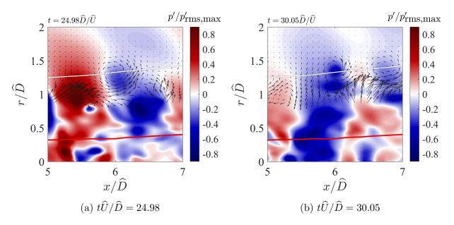
Figure 4.26: Contour of the instantaneous pressure fluctuation in jet AXI04U at  $\phi = 0^{\circ}$ . Arrows: projection of velocity fluctuation vectors on x - y plane; white line: radiator surface; red line: OSPS surface.
