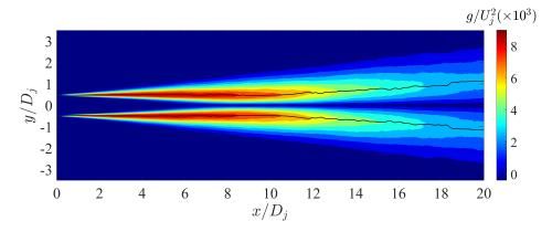
Figure 3.6: Isocontours of normalized Reynolds stress magnitude  $g/U_i^2$ . Black line: SPS.
