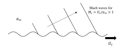
Figure 2.3: Mach wave emission in the case of a wavy wall moving with velocity  $U_c$  supersonic with respect to the ambient speed of sound.
