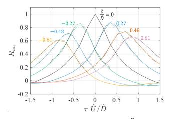
Figure 4.3: Space-time correlation  $R_{uu}$  on the OSPS at  $x/\hat{D} = 4$  for jet AXI04U. Dashed lines indicate fits by seventh-order polynomials to accurately detect the peak of each correlation.
