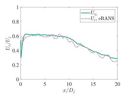
Figure 3.30: Comparison of LES- and eRANS-derived convective velocities on the radiator surface.
