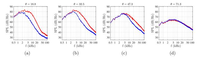
Figure 4.2: Far-field sound pressure level spectra of jets AXI04U (red) and ECC09U (blue) various polar angles  $\theta$  with respect to the downstream axis.
