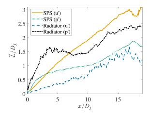
Figure 3.21: Axial distribution of length scales  $\hat{L}$  on the relevant surfaces. Orange solid line:  $\hat{L}_u$  on SPS. Blue dashed line:  $L_u$  on the radiator surface. Green dotted line:  $\hat{L}_p$  on the SPS. Black line dash-dot:  $\hat{L}_p$  on the radiator surface.
