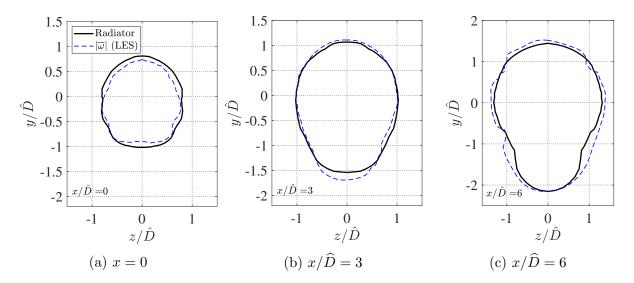
Figure 4.19: Comparison of radiator surface with surface based on the mean vorticity criterion of Eq. 4.4 using the LES flow fields on three cross-sectional planes of jet ECC09U.
