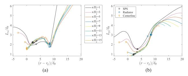
Figure 3.19: Plots of normalized length scales  $L/\delta_{\theta}$  versus normalized radius  $(r - r_i)/\delta_{\theta}$ , (a) based on axial velocity, (b) based on pressure. Legend applies to both subfigures.
