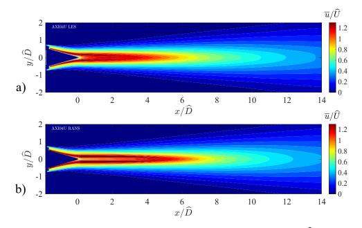
Figure 4.4: Isocontours of normalized normalized mean axial velocity  $\overline{u}/\hat{U}$  on the symmetry plane of jet AXI04U. a) LES and b) RANS.
