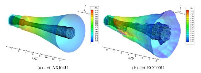
Figure 4.16: Radiator surfaces and LES-based OSPS with contours of convective Mach number  $M_c$ .
