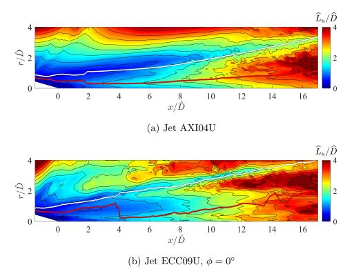
Figure 4.32: Isocontours of normalized moving-frame length scales based on axial velocity fluctuation,  $\hat{L}_u/\hat{D}$ . Red line: OSPS. White line: radiator surface.
