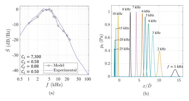
Figure 5.4: Results of model calibration to experimental far-field autospectra of jet AXI04U at  $\theta = 32.5^{\circ}$ . (a) Comparison of scaled experimental and modeled autospectra, and (b) real part of the axial distribution  $p_0(x)$ .
