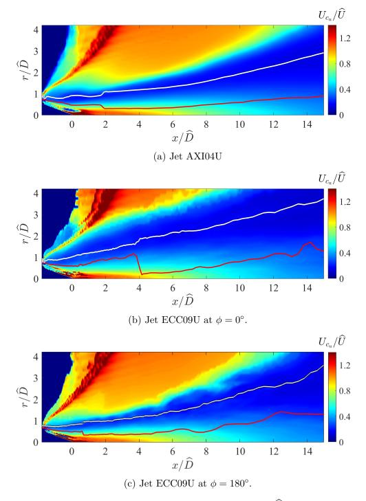
Figure 4.15: Distribution of normalized convective velocity  $U_{c_u}/\hat{U}$  on the meridional planes of jets AXI04U and ECC09U. The legend is the same as Fig. 4.14
