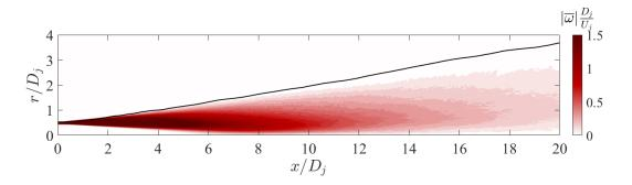
Figure 3.28: Isocontours of normalized magnitude of mean vorticity  $\overline{\omega}D_j/U_j$ . Black line: radiator surface based on  $U_c$ -match criterion.
