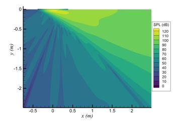
Figure A.4: Sound pressure levels generated from the short cylinder using a wavepacket of length scale  $L = 5\hat{D}$  along the vertical half-plane. The cylinder is visible near y = 0, spanning from x = -0.4 m to x = 0.4 m.
