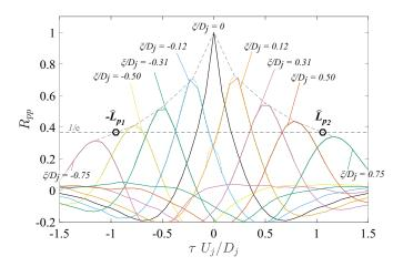
Figure 3.3: Space-time correlation  $R_{pp}$  in the vortical field at  $x/D_j = 2.5$  and  $r/D_j = 0.5$ . Dotted lines: fits by seventh-order polynomials. Dashed lines: envelope and ordinate relevant to the calculation of  $\hat{L}_p$ .
