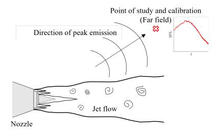
Figure 5.2: Sketch of noise radiation and point of study of the wavepacket model.
