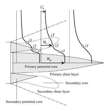
Figure 2.5: Basic elements of a two-stream jet, from Papamoschou [72].
