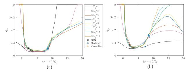
Figure 3.27: Azimuthal scales  $\Phi$  versus similarity coordinate  $(r - r_i)/\delta_{\theta}$ , (a) based on axial velocity; (b) based on pressure. Legend applies to both subfigures.
