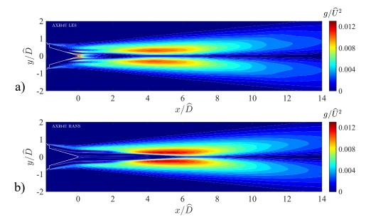
Figure 4.6: Isocontours of normalized Reynolds stress  $g/\hat{U}^2$  on a symmetry plane of jet AXI04U. a) LES and b) RANS.
