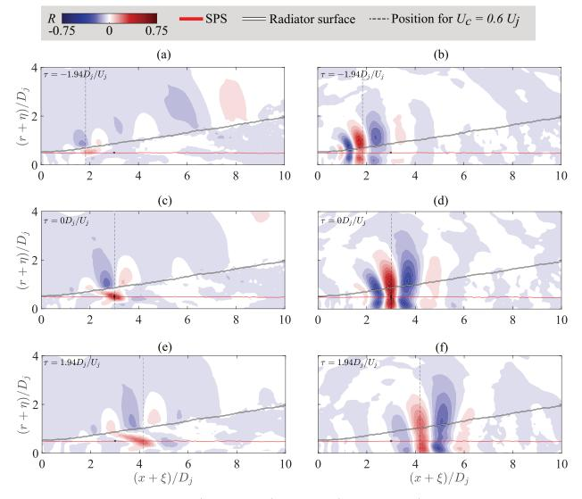
Figure 3.14: Contours of  $R_{uu}$  (left column) and  $R_{pp}$  (right column) with reference point on SPS at  $(x, r) = (3, 0.5)D_j$  for three time separations.
