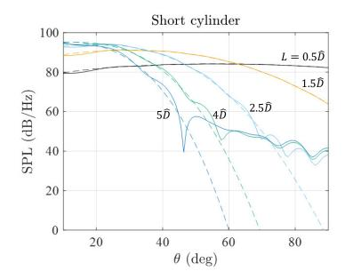
Figure A.3: Sound pressure levels from the standard cylinder BEM computation (solid lines) and the analytic formula (dashed lines) for polar angles  $\theta$  and wavepacket length scales L. Points are located at  $100\hat{D}$  from the origin.
