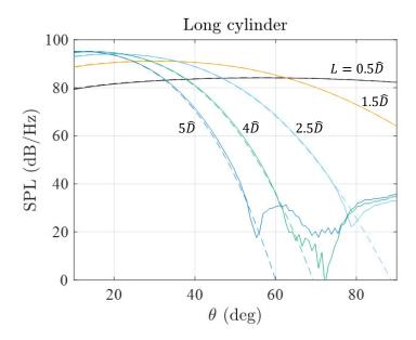
Figure A.5: Sound pressure levels from the long cylinder BEM computation (solid lines) and the analytic formula (dashed lines) for polar angles  $\theta$  and wavepacket length scales L. Field points are located at  $100\hat{D}$  from the origin.
