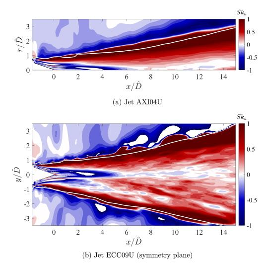
Figure 4.27: Distribution of the normalized skewness of the LES axial velocity field. White lines: radiator surface.
