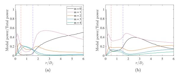
Figure 3.23: Radial distribution of modal powers on  $x = 7.5D_j$  for the first five modes; (a) based on axial velocity, (b) based on pressure. The vertical lines mark the locations of the SPS (red) and the radiator surface (blue).
