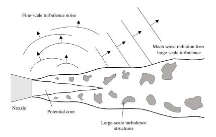
Figure 2.2: Diagram showing the turbulent mixing noise generation mechanisms in a single-stream jet.
