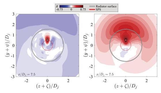
Figure 3.24: Contours of (a)  $R_{uu}$  and (b)  $R_{pp}$  on the cross-sectional plane  $x = 7.5D_j$  with reference point on SPS at  $\phi = \pi/2$  (white cross). Time shift is zero.
