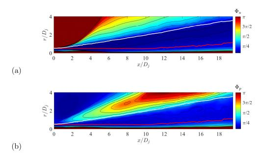
Figure 3.25: Isocontours of azimuthal scales (a)  $\Phi_u$  and (b)  $\Phi_p$ , units are radians. Red line: SPS. White line: radiator surface.
