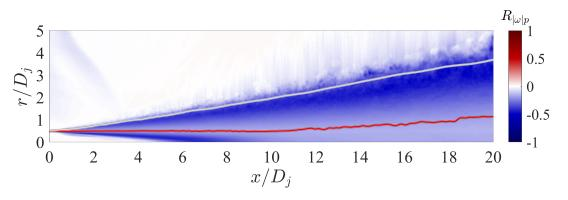
Figure B.4: Distribution of the normalized correlation between  $|\pm \omega|'$  and p',  $R_{|\pm \omega|p}$ . Red line: SPS. White line: radiator surface.
