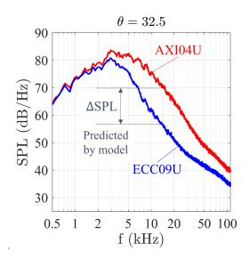
Figure 5.1: Far field SPL spectrum of jets AXI04U and ECC09U.
