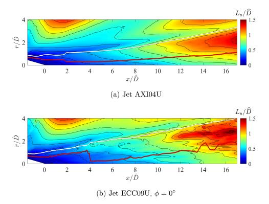
Figure 4.30: Isocontours of normalized fixed-frame length scales based on axial velocity fluctuation,  $L_u/\hat{D}$ . Red line: OSPS. White line: radiator surface.
