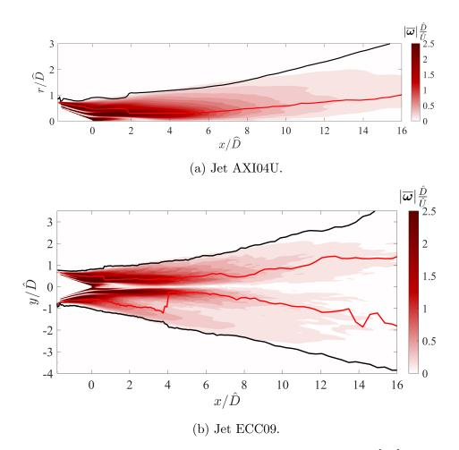
Figure 4.17: Isocontours of normalized module of mean vorticity  $|\overline{\boldsymbol{\omega}}| \widehat{D}/\widehat{U}$  on the meridional planes of jets AXI04U and ECC09U. Black line: radiator surface based on  $U_c$ -match criterion. Red line: OSPS
