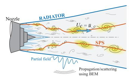
Figure 2.7: Representation of the wavepacket model for a multi-stream jet.
