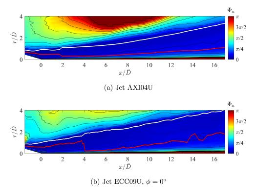
Figure 4.36: Isocontours of azimuthal scales based on axial velocity fluctuation,  $\Phi_u$ . Red line: OSPS. White line: radiator surface.
