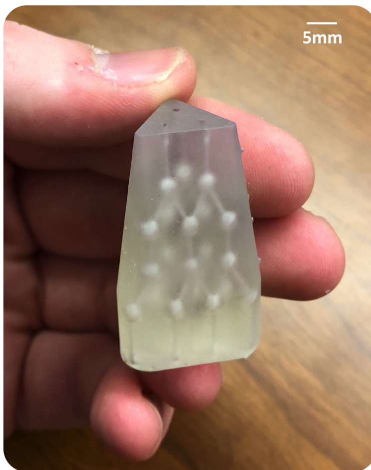
Figure 3.15: Fabrication results, tetrahedral -based 3D \mu -CGG device after post-processing revealing hollow microchannel structures visible through the translucent material comprising the body of the device. The prototype is shown held between this Doctoral Candidate researcher's fingers, for scale.
