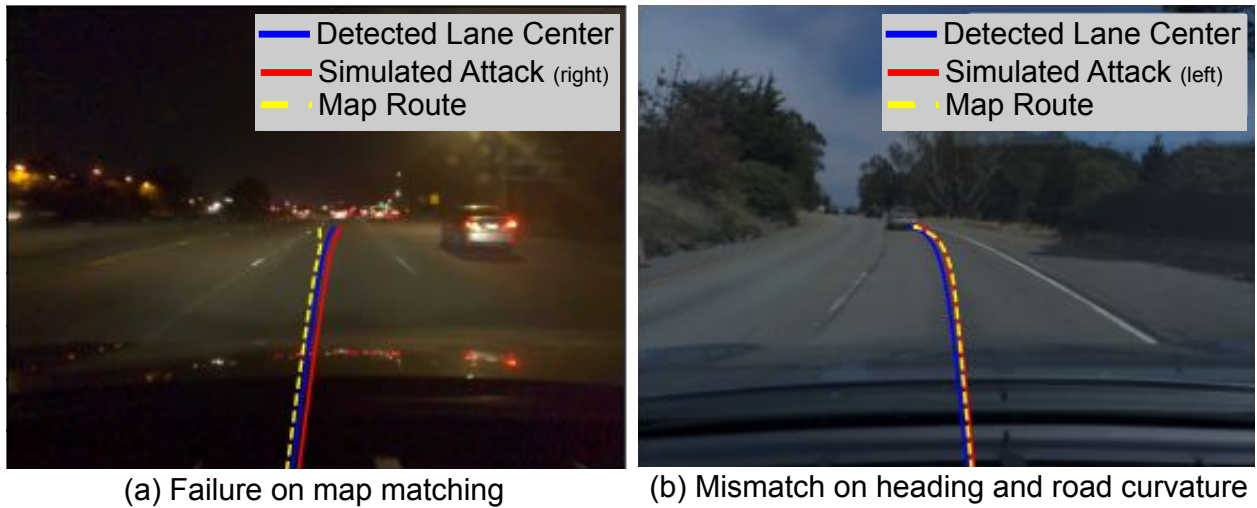
Figure 4.3.3: Case studies on false positives: (a) The map is associated with the wrong point as the road curve should start at a further point; (b) the vehicle heading does not match with the road curvature while the detected lane center looks accurate.
