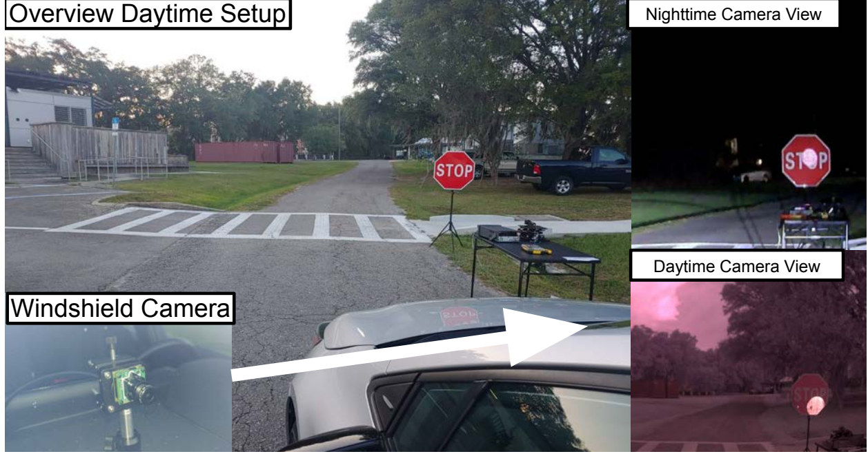
Figure 6.5.5: Overview of the outdoor experimental scenarios. The setup is used in the daytime (left). The camera view during the attack is at nighttime (Right-top) and daytime (Right-bottom).
