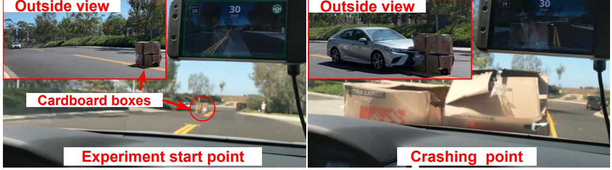
Figure 3.14: Safety impact evaluation for our attack on a Toyota 2019 Camry with OpenPilot engaged. Even with other driver assistance features such as Automatic Emergency Braking (AEB), our attack still causes collisions in all the 10 trials.
