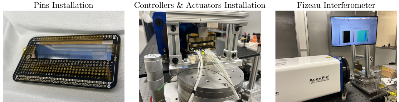
Figure 7. Experimental setup for the measurement of thin adaptive optics segment 3A at the University of Iowa.
