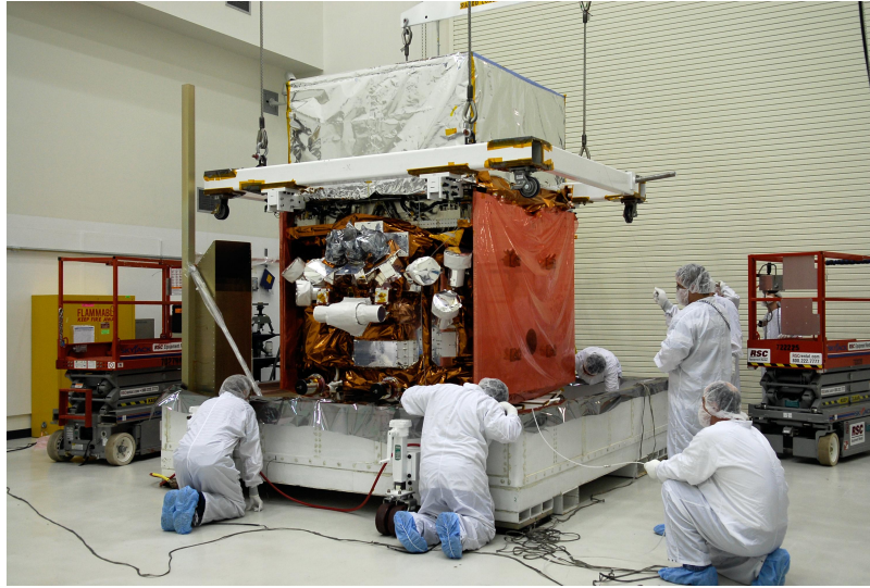
Figure 3.1: Engineers inspect the Fermi spacecraft. GBM detectors are visible in white on the front facing portion. The LAT is the silver portion on the top of the satellite. The white frame surrounding the satellite is a crane, and not part of the Fermi telescope.
