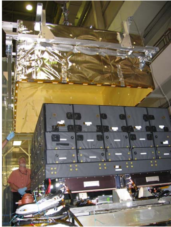
(a) The ACD (black), with micrometeorite shield (gold) suspended above. Image Credit: Diane Schuster / NASA
