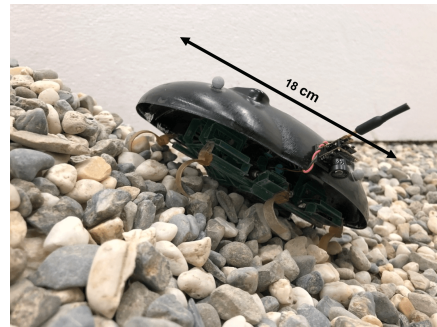
Figure 3.2: VelociRoACH: our small, mobile, highly dynamic, and bio-inspired hexapedal millirobot, shown with a camera mounted for terrain imaging.
