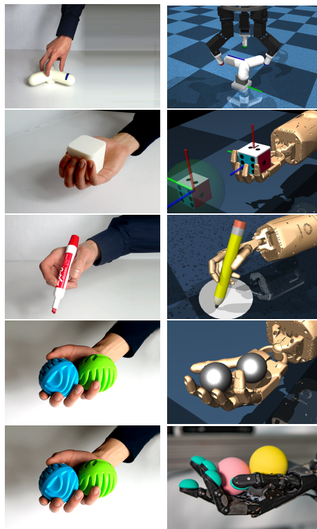
Figure 4.3: Task suite of simulated and real-world dexterous manipulation: valve rotation, in-hand reorientation, handwriting, and manipulating Baoding balls.
