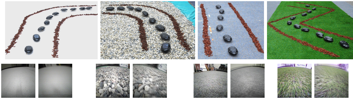
Figure 3.13: Top: Execution of our model-based learning method, using an image-conditioned dynamics model, on various desired paths on four terrains (styrofoam, gravel, carpet, and turf). Note that the path boundaries are outlined for visualization purposes only, and were not present during the experiments. Bottom: Example images from the onboard camera during the runs (shaky images due to body motion).
