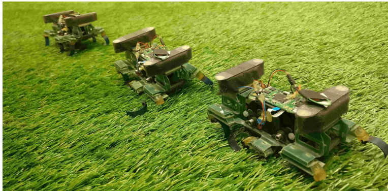
Figure 5.2: We implement our sample-efficient meta-reinforcement learning algorithm on a real legged millirobot, enabling online adaptation to new tasks and unexpected occurrences such as losing a leg (shown here), novel terrains and slopes, errors in pose estimation, and pulling payloads.
