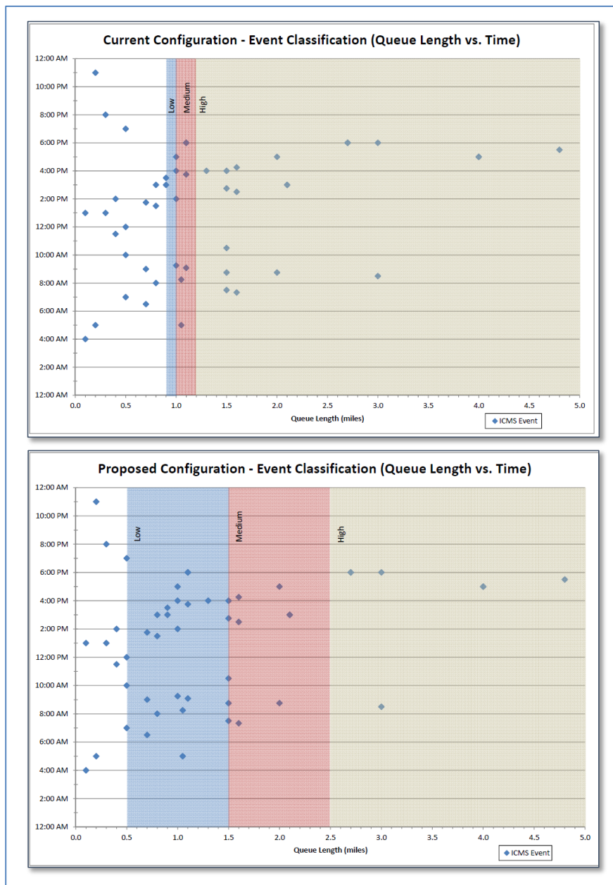
Figure 7-52 – Effect of Queue Threshold Change on Low-, Medium-, or High-Impact Event Classification
