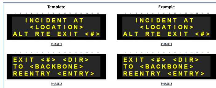
Figure 7-37 – Initial Template for Routing Information on Freeway CMSs
