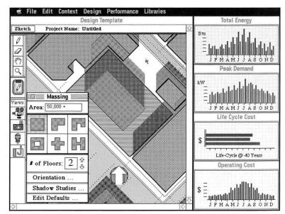
**Figure 2.** Through a Schematic Design Tool that incorporates shadow-casting visualization, EDA will assist building designers with initial building massing and orientation decisions, providing feedback on multiple performance considerations.
