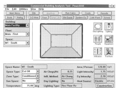
**Figure 3.** The interactive user interface of PowerDOE allows a designer to specify the various building components and systems easily while providing visual feedback on the placement of building envelope elements in plan and elevation views.
