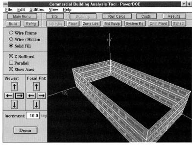
*Figure 1. PowerDOE includes a user-controlled, three-dimensional perspective and axonometric display of the whole building configuration.*
