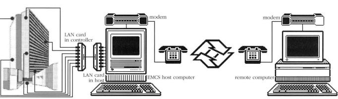
Although there is a wide range in EMCS characteristics, most current- and next-generation EMCSs contain sensors, sophisticated networking hardware, data-storage algorithms, and communications hardware and software, all of which make the EMCS an ideal platform for commercial building performance monitoring.
