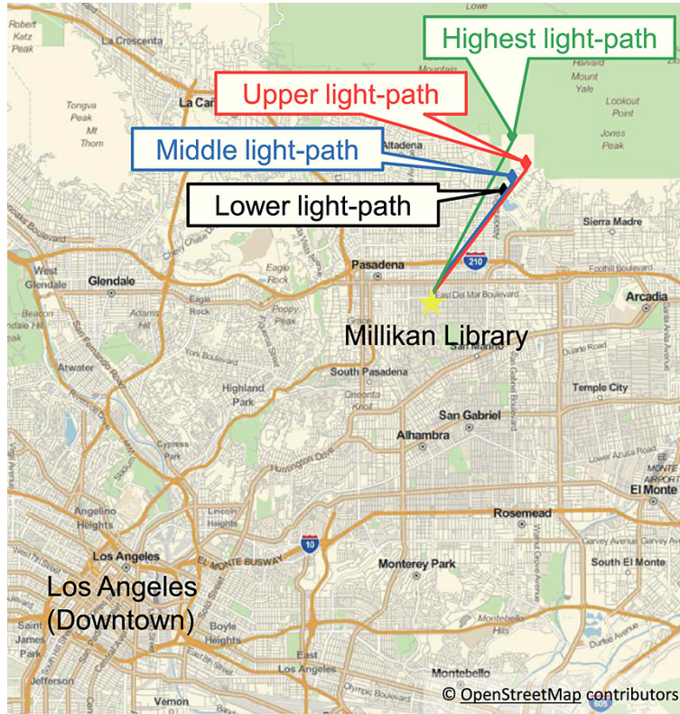
Figure 2.1: Map of the CalNex Pasadena ground site, shown with a star, in relation to downtown Los Angeles. The LP-DOAS retroreflector array locations and light paths are also shown in the colored diamonds and lines. Figure from Tsai et al. (2014).
