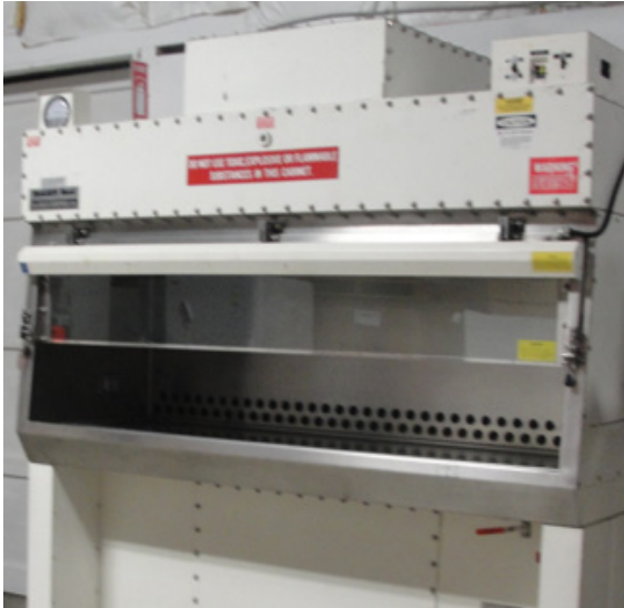
Figure 4: Biogard Biosafety Hood. The airflow is inward protecting the person working with infectious materials.
