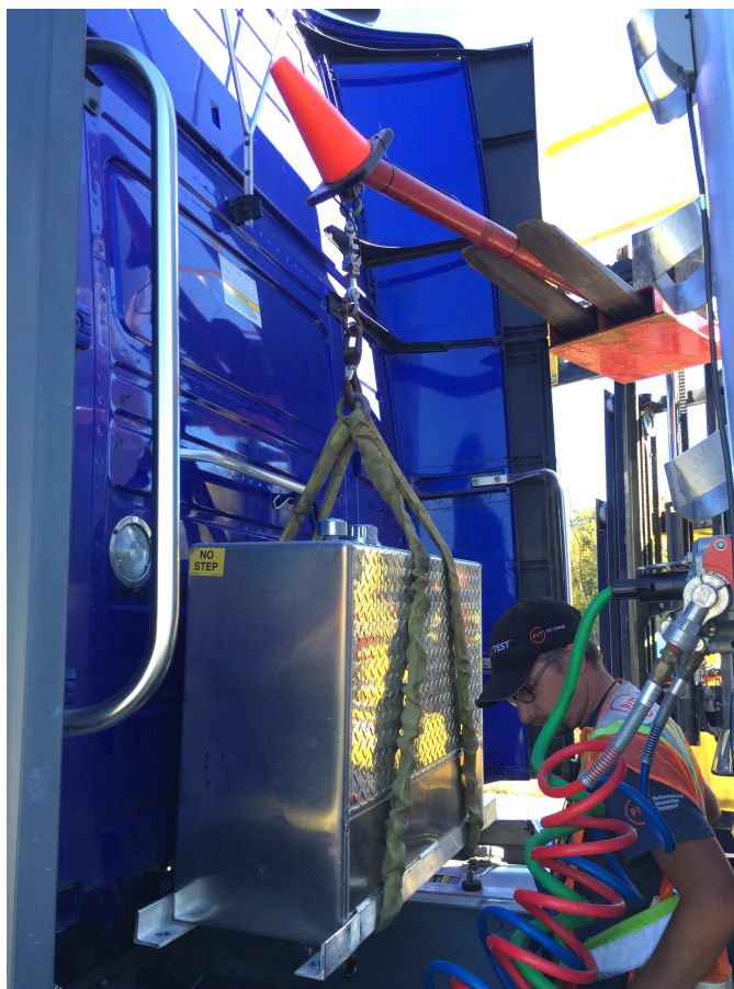
Figure 2.8: Photograph of auxiliary fuel-tank weighing procedure.
