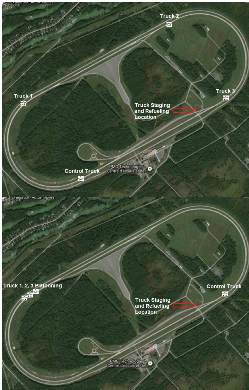
Figure 2.5: Satellite photograph of the test track (top - vehicle configuration for independent-vehicle test runs, bottom - vehicle configuration for platooning test runs).
