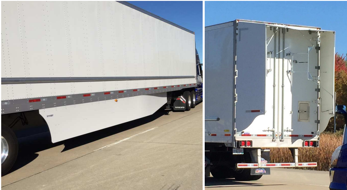
Figure 2.4: Photograph of side-skirts and boat-tail installed for the aerodynamic-trailer test configuration.
