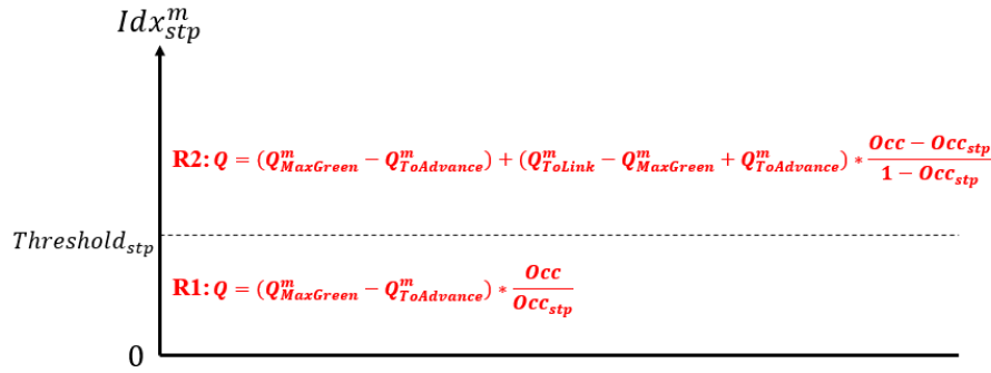
Figure 29 Calculation of vehicle queues with only stoplevel detectors.
