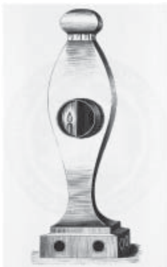
Fig. 8. The “lichtleiter” or light conductor of Bozzini. One can see the candle used for illumination immediately next to the eyepiece for viewing.
