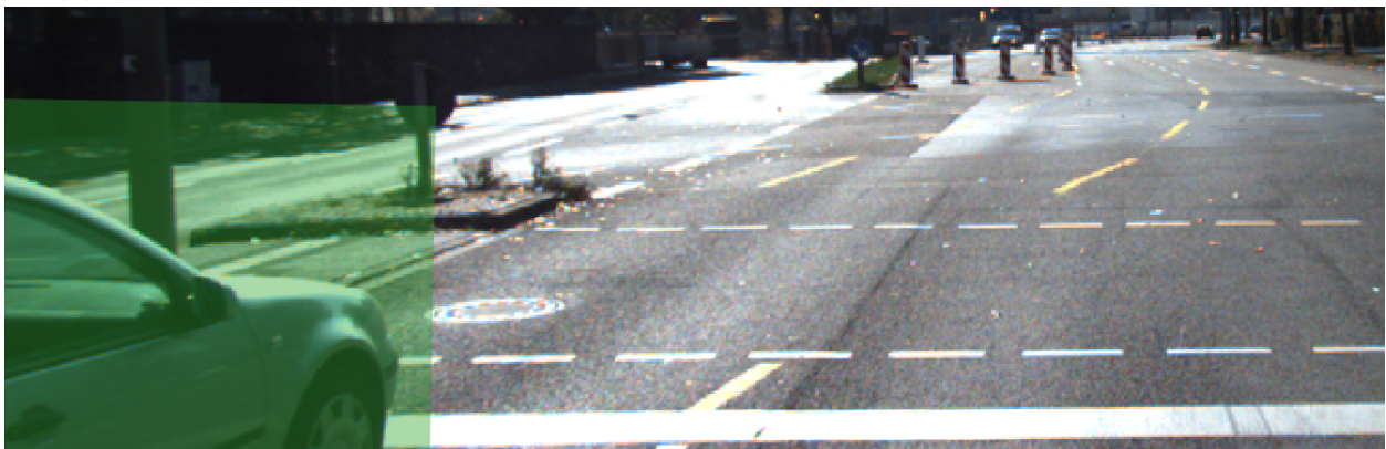
(c) 2D bounding box is located at the boarder of image. This makes it difficult to apply geometrical agreement search.
