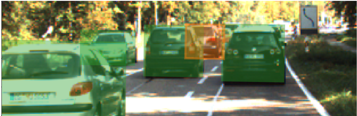
(a) Object missed from 2D camera detector. Yellow box is false negative which is missed from the 2D detector.
