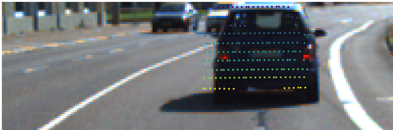
(b) asynchronization between camera and LiDAR timestamp
