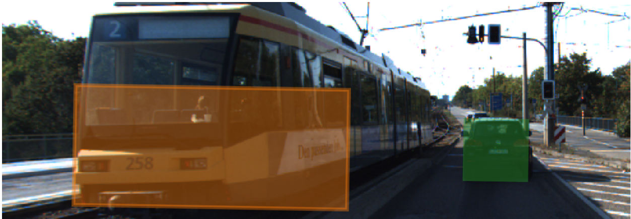
(b) Tram is classified as vehicle. Yellow box is false positive detection from the 2D detector
