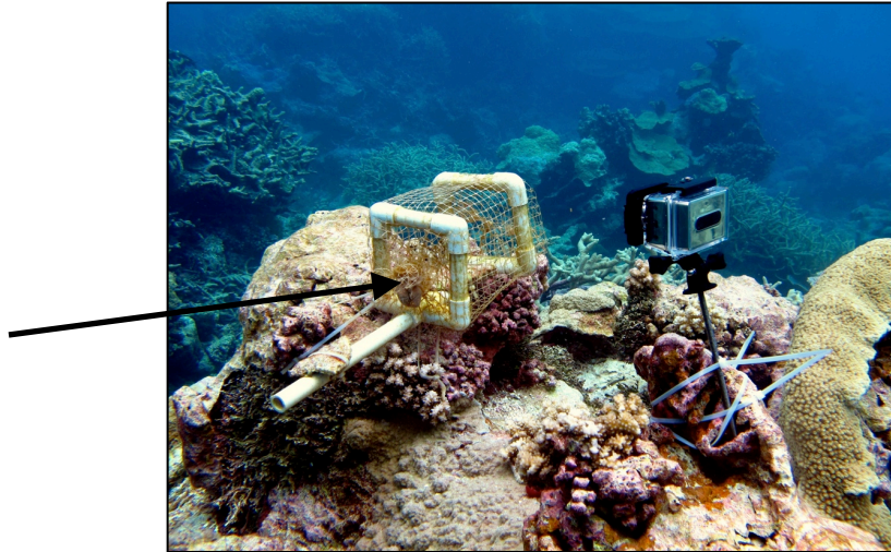
Figure 3.2 Experimental setup with plates of dead coral covered in turf algae placed outside and inside mesh cages. Arrow indicates nylon mesh bag containing fertilizer located equidistant from turf inside and outside cage as part of the nutrient addition treatment.
