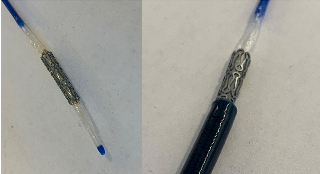
Figure 74: Version 3 stent tightly attached on the ballon
