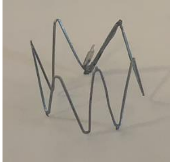
Figure 60: Expanded V1 stent
