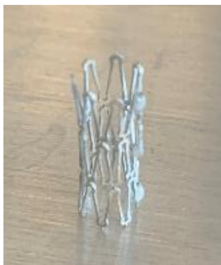
Figure 64: Successfully deployed stent using 8 mm balloon
