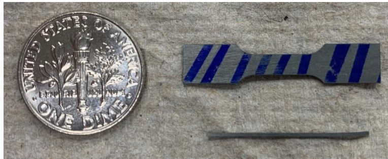
Figure 53: Tensile and fatigue test specimen
