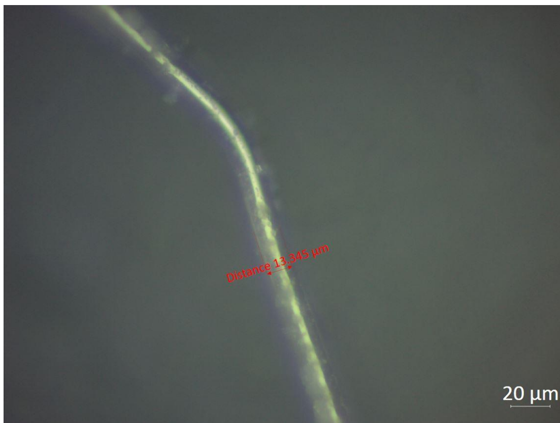
Figure 102: Optical microscopy image of Ag microwire by thermal fiber drawing
