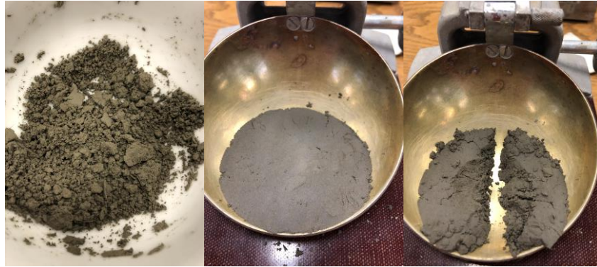
Figure C.2.1. Soil is too dry so its liquid limit cannot be determined using the Casagrande's method.
