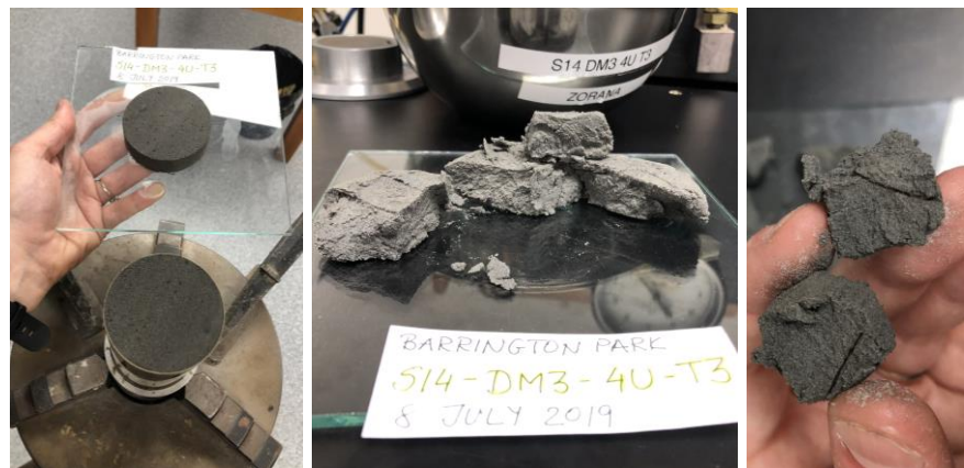
Figure D.1.20. S14-DM3-4U-T3 before and after CSS testing.
