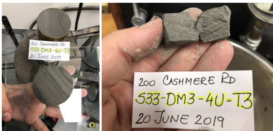
Figure D.1.33. S33-DM3-4U-T3 before and after CSS testing.
