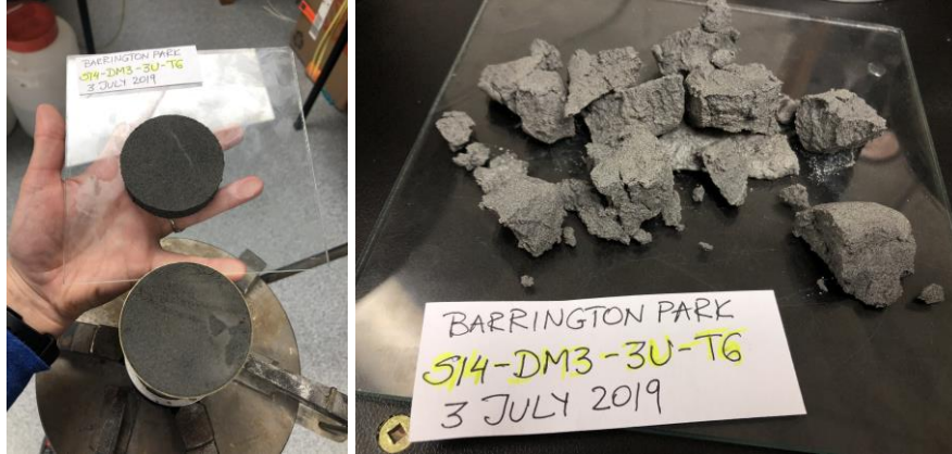
Figure D.1.16. S14-DM3-3U-T6 before and after CSS testing.
