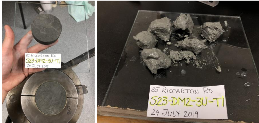
Figure D.1.37. S23-DM2-3U-T1 before and after CSS testing.
