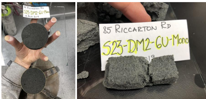
Figure D.1.9. S23-DM2-6U-M before and after MSS testing.
