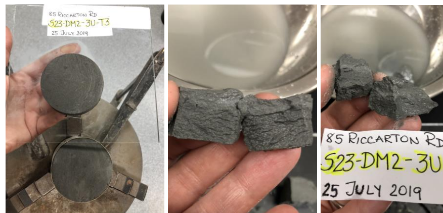
Figure D.1.39. S23-DM2-3U-T3 before and after CSS testing.
