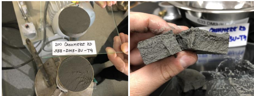
Figure D.1.28. S33-DM3-3U-T4 before and after CSS testing.
