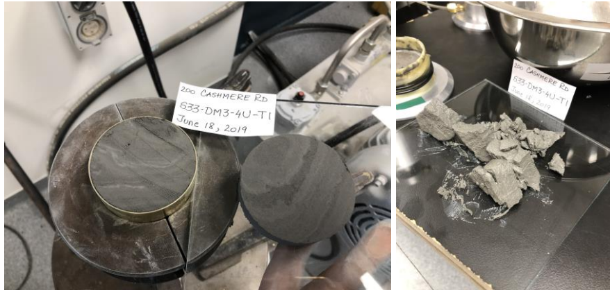
Figure D.1.31. S33-DM3-4U-T1 before and after CSS testing.
