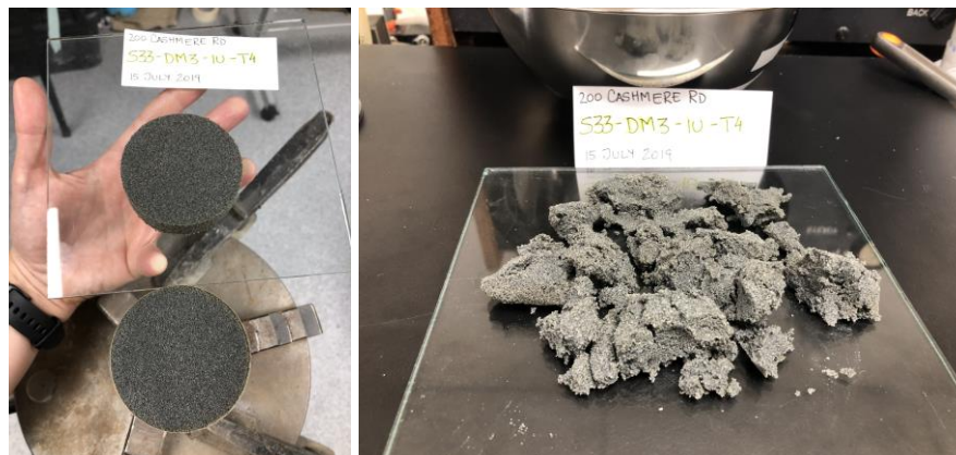
Figure D.1.3. S33-DM3-1U-T4 before and after CSS testing.
