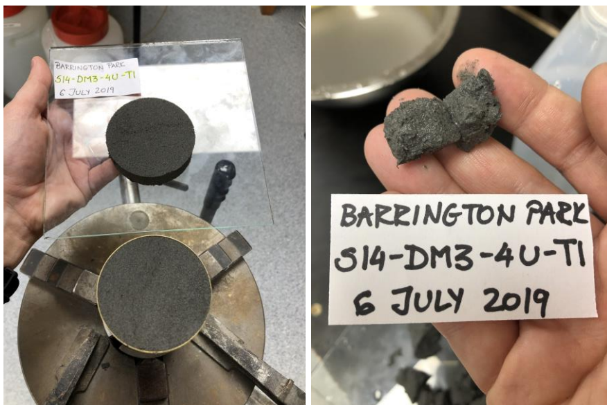
Figure D.1.18. S14-DM3-4U-T1 before and after CSS testing.
