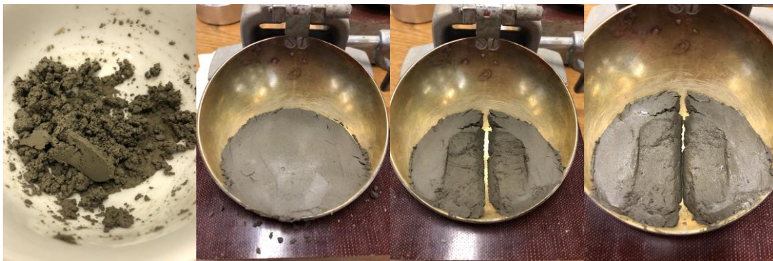
Figure C.2.2. Soil is at its plastic limit yet above its liquid limit according to the Casagrande's method.
