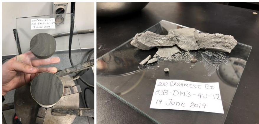
Figure D.1.32. S33-DM3-4U-T2 before and after CSS testing.
