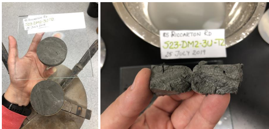
Figure D.1.38. S23-DM2-3U-T2 before and after CSS testing.
