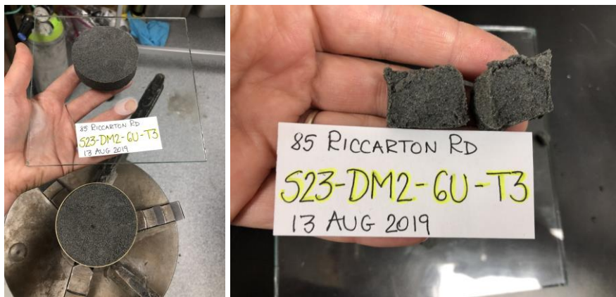
Figure D.1.8. S23-DM2-6U-T3 before and after CSS testing.
