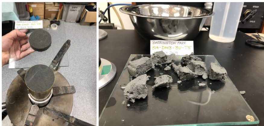
Figure D.1.15. S14-DM3-3U-T5 before and after CSS testing.
