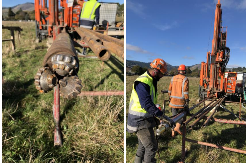
Figure B.3.1. Tri-cone roller bit and thin-walled brass tube attached to the Dames and Moore sampler.
