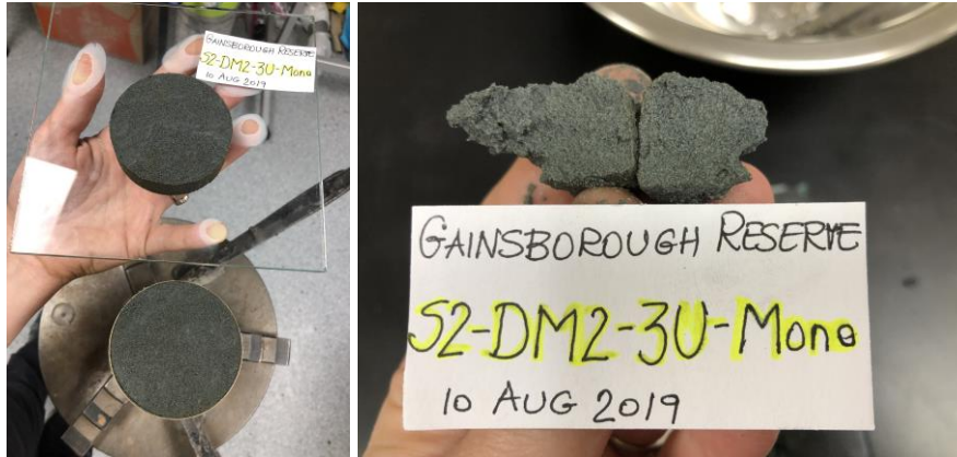
Figure D.1.13. S2-DM2-3U-M before and after MSS testing.
