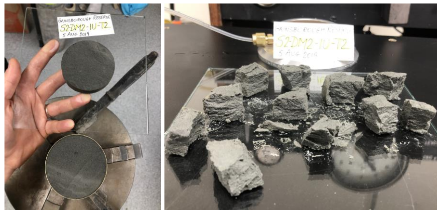
Figure D.1.35. S2-DM2-1U-T2 before and after CSS testing.
