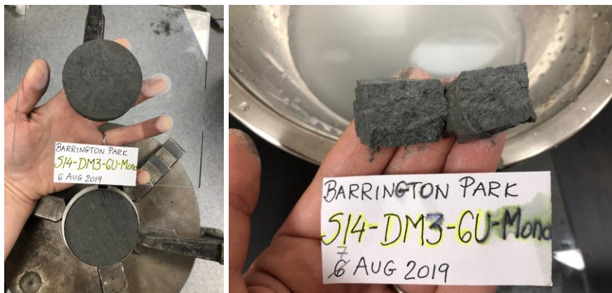
Figure D.1.27. S14-DM3-6U-M before and after MSS testing.
