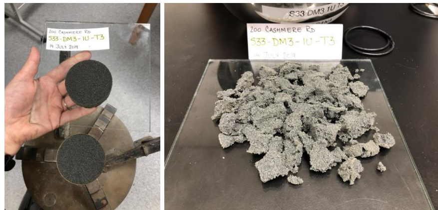
Figure D.1.2. S33-DM3-1U-T3 before and after CSS testing.
