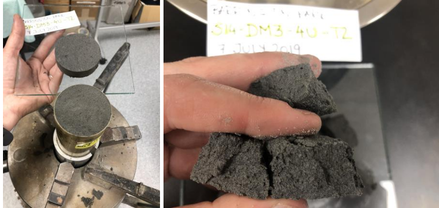
Figure D.1.19. S14-DM3-4U-T2 before and after CSS testing.
