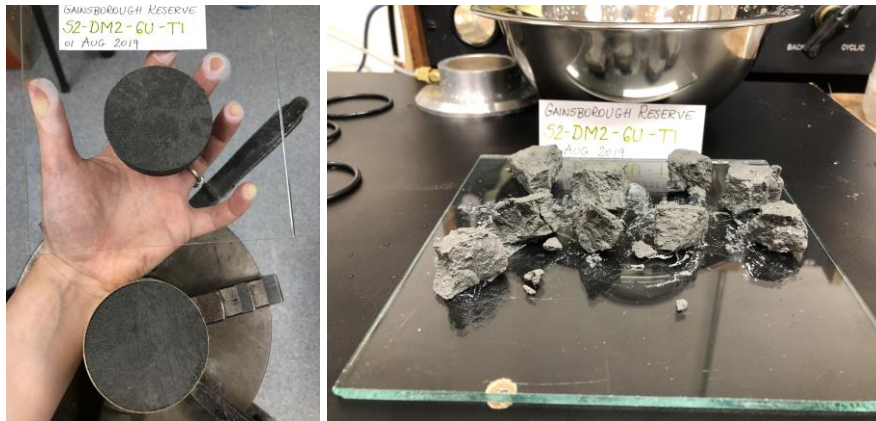
Figure D.1.22. S2-DM2-6U-T1 before and after CSS testing.
