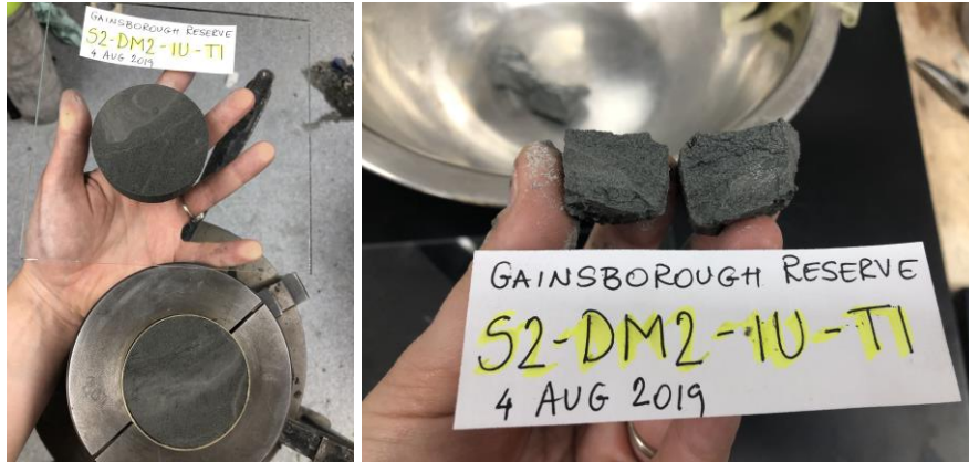
Figure D.1.34. S2-DM2-1U-T1 before and after CSS testing.
