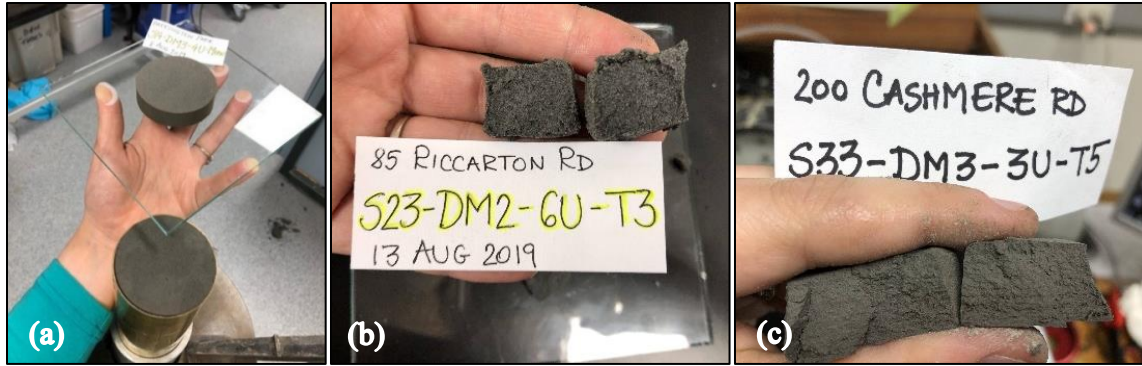
Figure 5.3. Test specimen appearance: (a) S14-DM3-4U-M (ML) before testing, (b) S23-DM2-6U-T3 (SM) after testing, and (c) S33-DM3-3U-T5 (ML) after testing.
