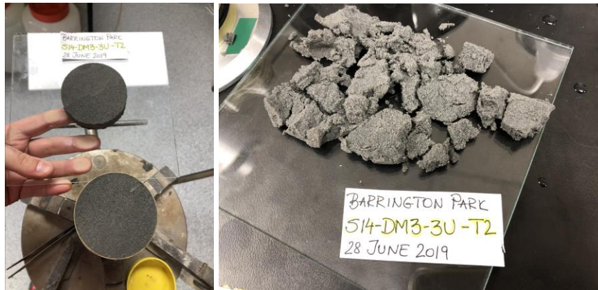
Figure D.1.41. S14-DM3-3U-T2 before and after CSS testing. This test specimen is not presented in Chapter 5.
