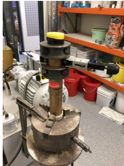
Figure B.3.2. Brass tube cutting prior to soil extrusion.
