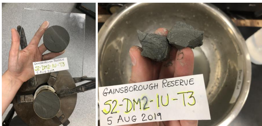
Figure D.1.36. S2-DM2-1U-T3 before and after CSS testing.
