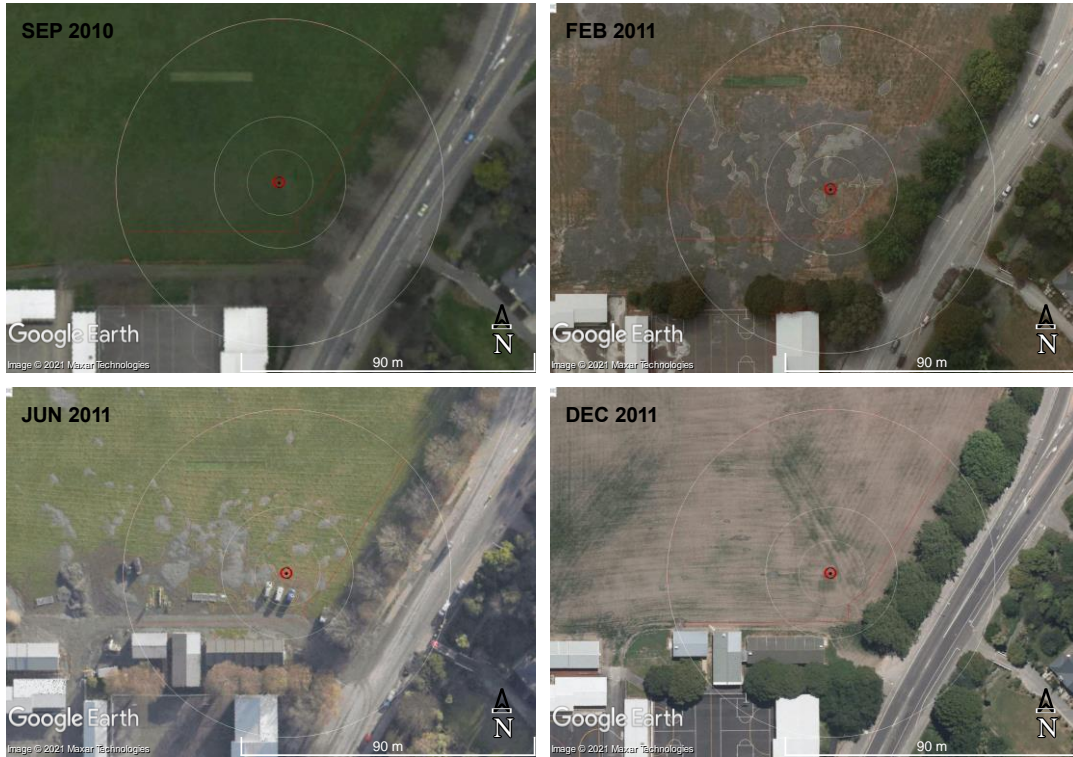
Figure 2.6. Aerial photographs acquired for Shirley Intermediate School in Sep 2010, Feb 2011, Jun 2011, and Dec 2011 (CGD 2012a) with ejecta outlines for the 10-, 20-, and 50-m buffers.
