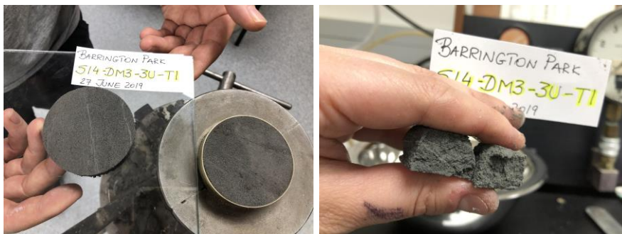
Figure D.1.14. S14-DM3-3U-T1 before and after CSS testing.
