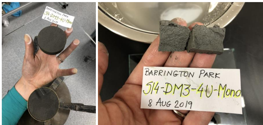
Figure D.1.21. S14-DM3-4U-M before and after MSS testing.
