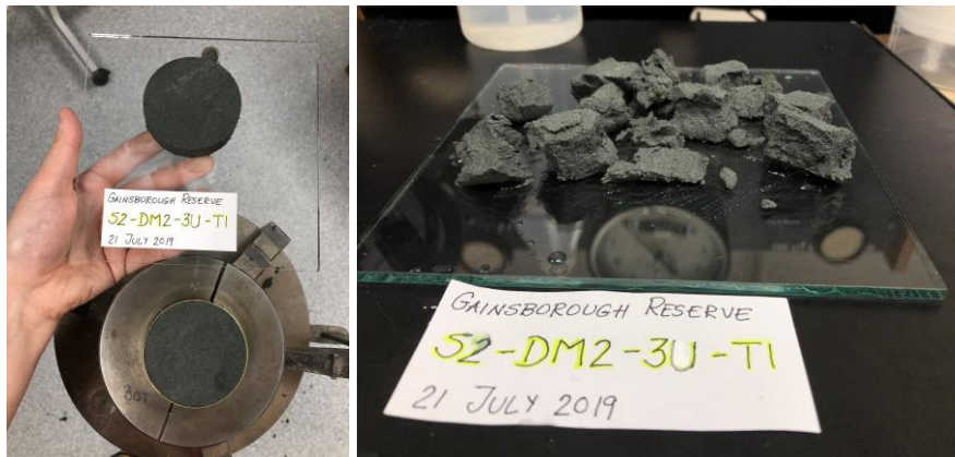
Figure D.1.10. S2-DM2-3U-T1 before and after CSS testing.
