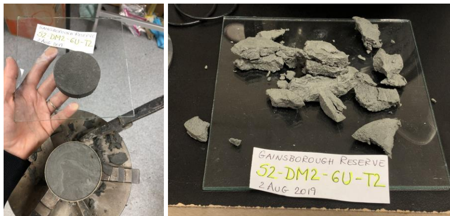
Figure D.1.23. S2-DM2-6U-T2 before and after CSS testing.
