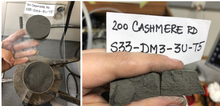
Figure D.1.29. S33-DM3-3U-T5 before and after CSS testing.
