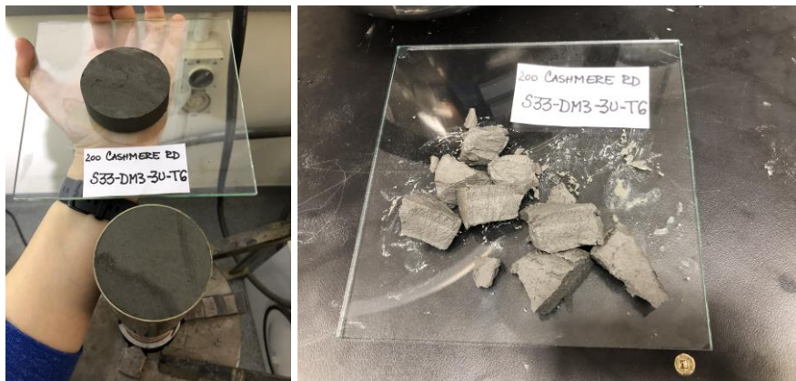
Figure D.1.30. S33-DM3-3U-T6 before and after CSS testing.
