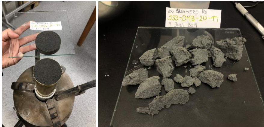
Figure D.1.5. S33-DM3-2U-T1 before and after CSS testing.
