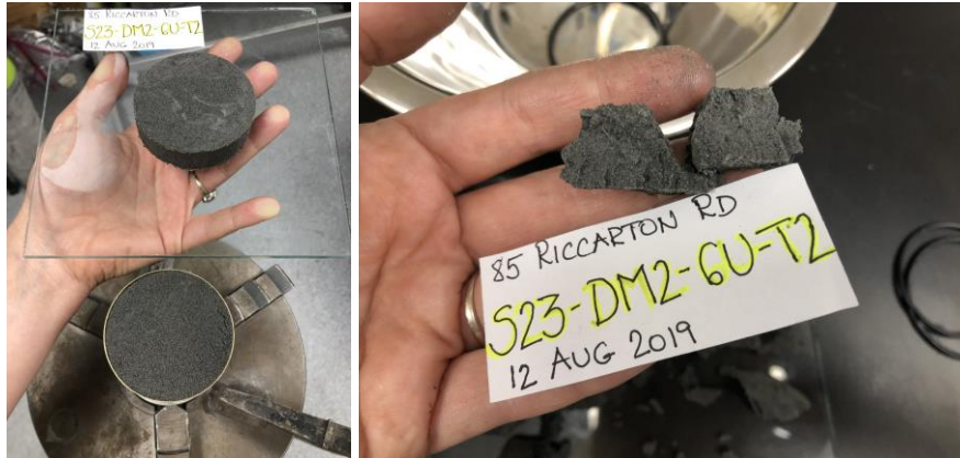
Figure D.1.7. S23-DM2-6U-T2 before and after CSS testing.
