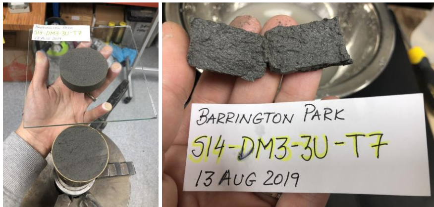
Figure D.1.17. S14-DM3-3U-T7 before and after CSS testing.
