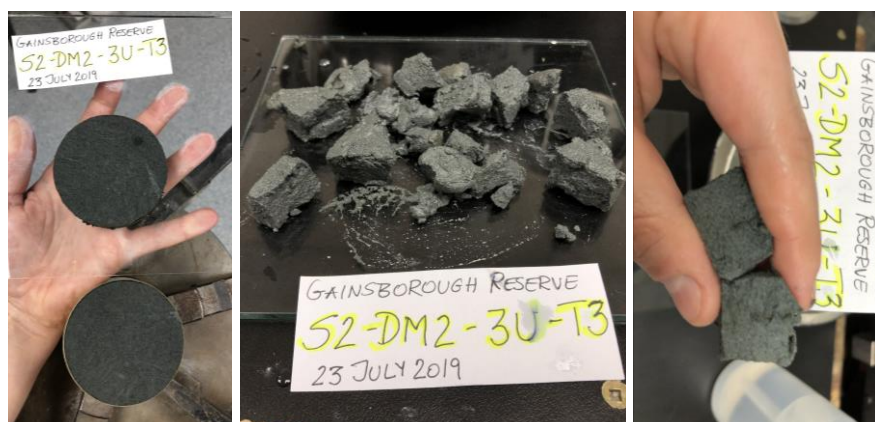
Figure D.1.12. S2-DM2-3U-T3 before and after CSS testing.
