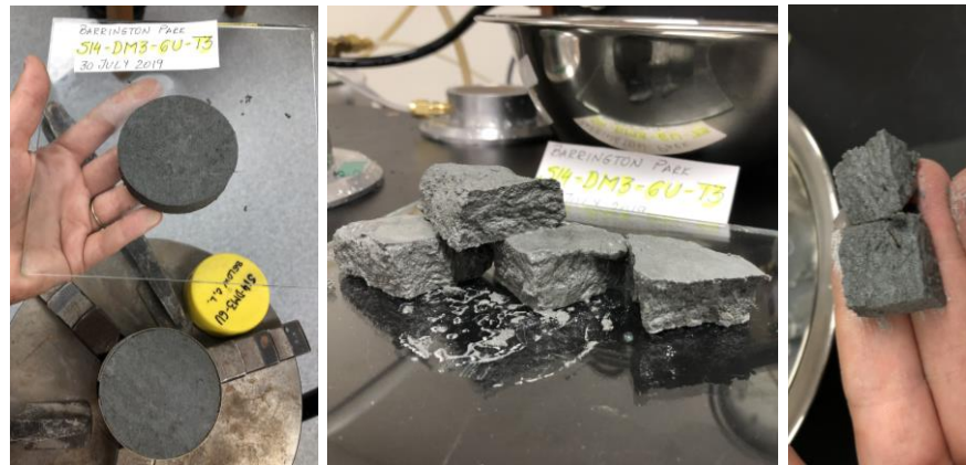
Figure D.1.26. S14-DM3-6U-T3 before and after CSS testing.
