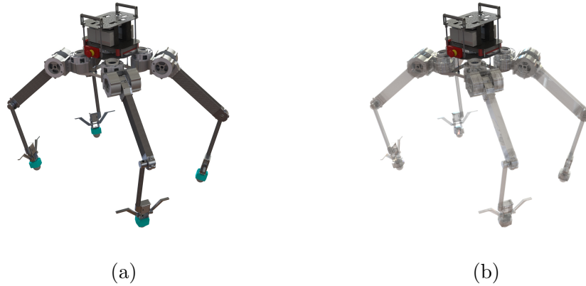
Figure 4.6: a) Pose of the robot that was used to approximate the inertia tensor assuming the entire robot as a single rigid body. b) The solid part representing the actual inertia that should be considered for the rotation about the Z axis.
