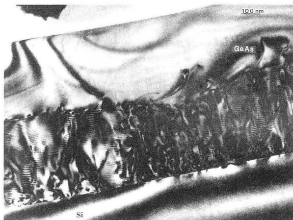
Figure 1 TEM cross-section micrograph of the GaAs/Si interface with 50 periods of InGaAs (25% In)/GaAs strained layer superlattices (SLSL) grown directly at the interface with Si. Note the large number of stacking faults formed at the interface, propagating through the SLSL and stopping at the last interface with epilayer of GaAs. Bending of dislocations was most effective at this interface. XBB 871-46
