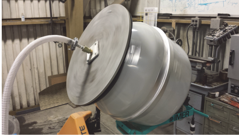
Figure 64 – Electric mixing chamber available at the facility
