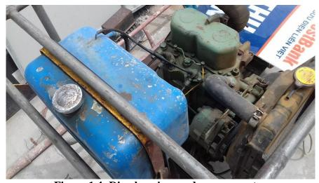
Figure 1.4: Diesel engine used as a generator
