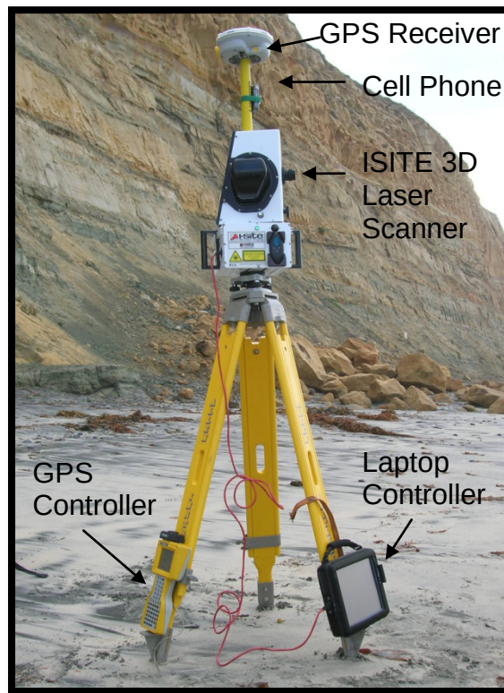
Figure 4-2. Field survey equipment and setup
