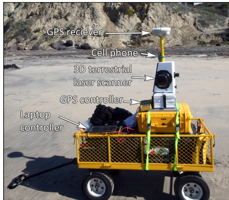
Figure 2-3. Terrestrial laser scanner and RTK GPS field equipment
